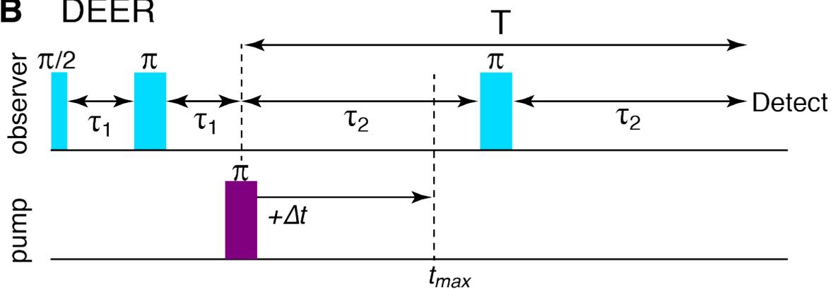
**Figure S1.** Pulse schemes for (A) two-pulse Hahn spin echo and (B) four-pulse DEER<sup>8</sup> experiments. In the current work, the duration of the blue  $\pi/2$  and  $\pi$  pulses are 12 and 24 ns, respectively, and that of the purple  $\pi$  pulse is 10 ns.
