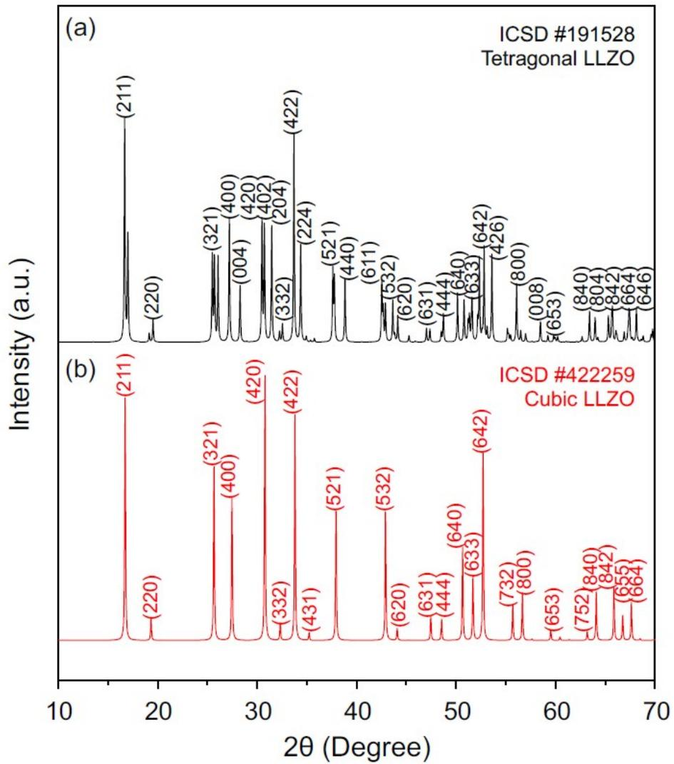
**Figure S2.** XRD patterns with indexing the planes of (a) tetragonal and (b) cubic phase LLZO.
