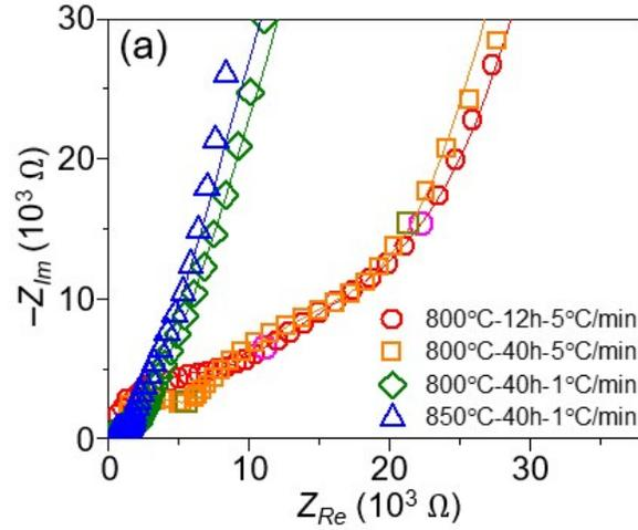
**Figure S5.** A Nyquist plot of the B-Al-LLZO samples with different heating conditions. EIS was measured in 7 MHz – 3 kHz at room temperature.
