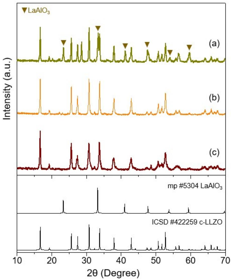
**Figure S3.** XRD patterns of Al-doped LLZO with (a)  $\text{AlPO}_4$  10 wt%, (b)  $\text{Li}_3\text{PO}_4$  10 wt% and (c)  $\text{Li}_3\text{BO}_3$  10 wt% obtained by first and second heat treatment at  $600^\circ\text{C}$  and  $800^\circ\text{C}$  for 12 h and subsequently heat treated at  $800^\circ\text{C}$  for 12 h at high cooling rate ( $5^\circ\text{C}/\text{min}$ )
