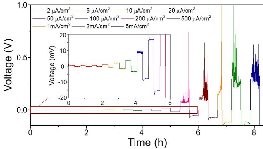
**Figure S6.** The voltage polarization profile of the Li symmetric cell of B-Al-LLZO sintered at 850°C for 40 h with 1°C/min cooling at room temperature as a function of applied current density ranging from 2  $\mu\text{A}/\text{cm}^2$  to 5  $\text{mA}/\text{cm}^2$ .
