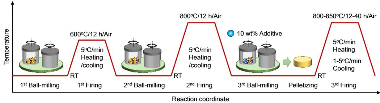
**Figure S1.** Schematic illustration of the LLZO preparation procedure in this work.
