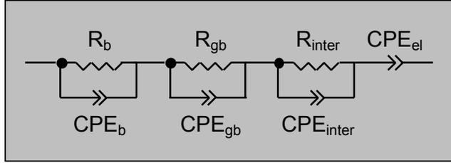
**Figure S4.** Equivalent circuit to model impedance of bulk (b), grain boundary (gb), and interphase (inter).
