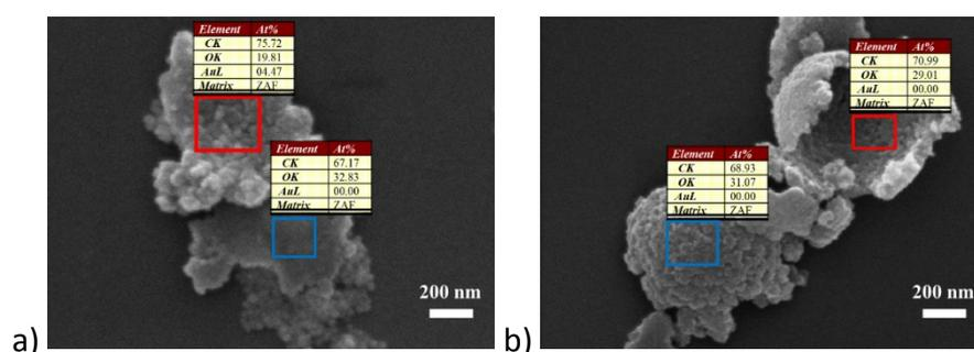
**Figure S6.** SEM images and inset EDX results of the fragments of the two different Janus cages: (a) PNIPAM-cPVBC-PEO; (b) cPVBC-PEO.
