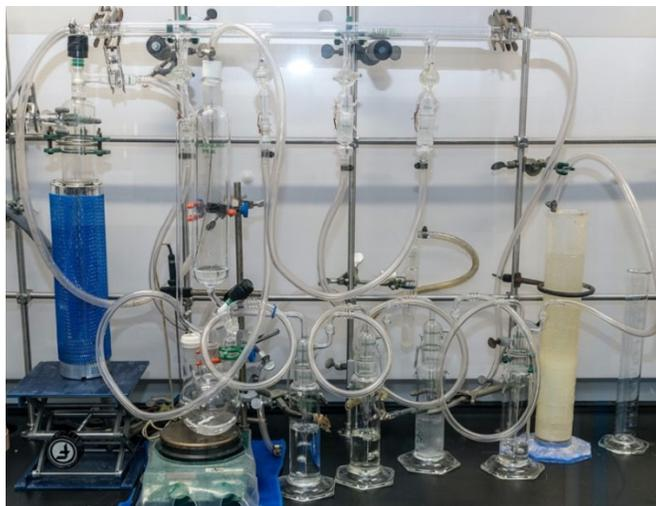
**Figure S1.** Assembled glassware for synthesis and purification of COS.
