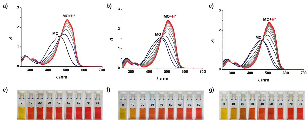
**Figure S14.** UV/Vis spectral titration for methyl orange (**MO**) as a pH indicator using 0.05 M HCl and its photographs: (a) and (e) only deionized water, the solution containing lithium carbonate extracted by (b) and (f) 20 mg of **1**, (c) and (g) 40 mg of **1**.
