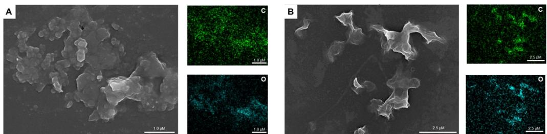
**Figure S17.** The images of SEM/EDS mapping of oxygen and carbon for A) commercial lithium carbonate and B) lithium carbonate extracted by **1**.
