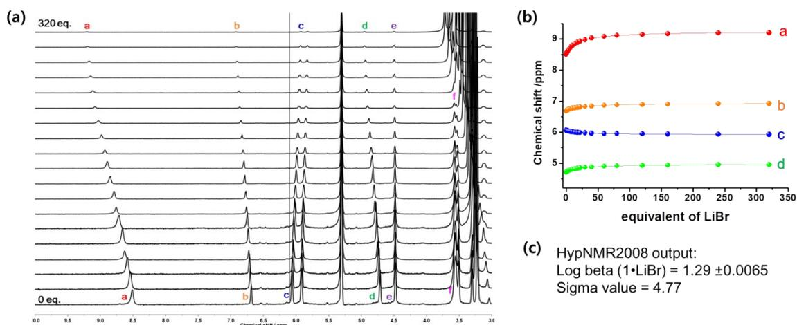
**Figure S5.** (a) stacked partial  $^1\text{H}$  NMR spectra of **1** (10 mM) with LiBr in 10%  $\text{CD}_3\text{OD}/\text{CD}_2\text{Cl}_2$ , (b) chemical shift changes of **1**'s protons upon addition of LiBr, (c) binding constant of **1**• LiBr calculated by HypNMR2008.
