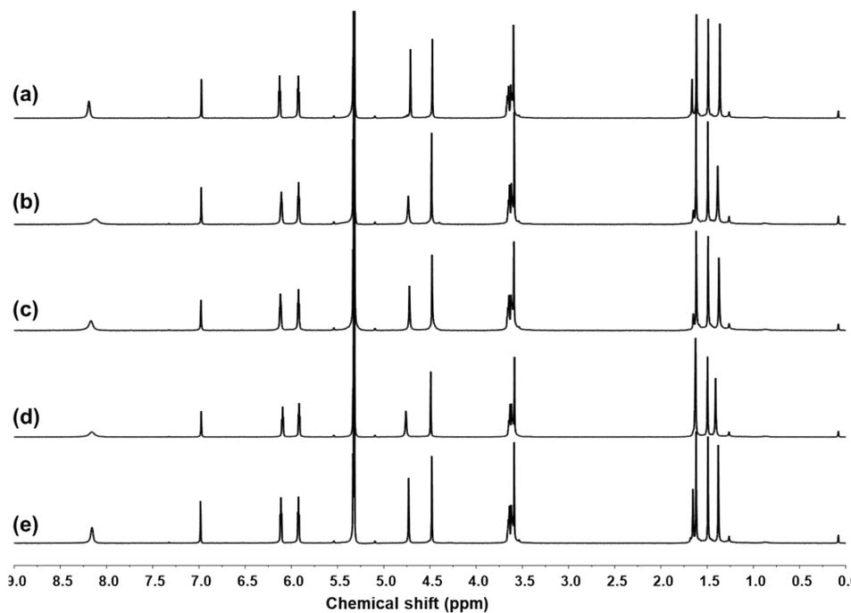
**Figure S12.**  $^1\text{H}$  NMR spectra of (a) **1** (5 mM) and **1** after extraction with excess of (b) NaCl(aq), (c) KCl(aq), (d) NaBr(aq), and (e) KBr(aq) (all spectra were recorded  $\text{CD}_2\text{Cl}_2$ , 297 K).
