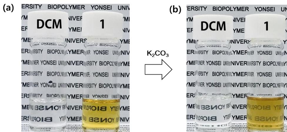
**Figure S16.**  $\text{Li}_2\text{CO}_3(\text{s})$  was precipitated by addition of  $\text{K}_2\text{CO}_3$  diluted in methanol into the solution containing **1**•LiCl complex; (a) before addition of  $\text{K}_2\text{CO}_3$  and (b) after addition of  $\text{K}_2\text{CO}_3$ .
