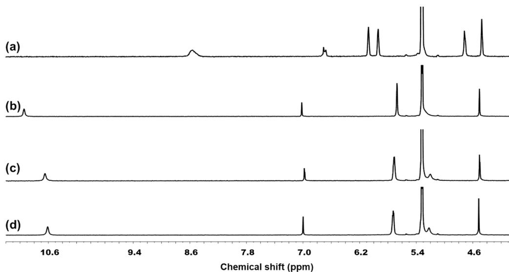
**Figure S2.** Partial  $^1\text{H}$  NMR spectra to confirm complexation of **1**•LiCl in solution state. (a) only **1** (10 mM) and **1** with (b) excess of TBACl, (c) TBACl followed by excess of LiClO<sub>4</sub>, (d) excess of LiCl. (all spectra were recorded in 10% CD<sub>3</sub>OD/CD<sub>2</sub>Cl<sub>2</sub>, 297 K)
