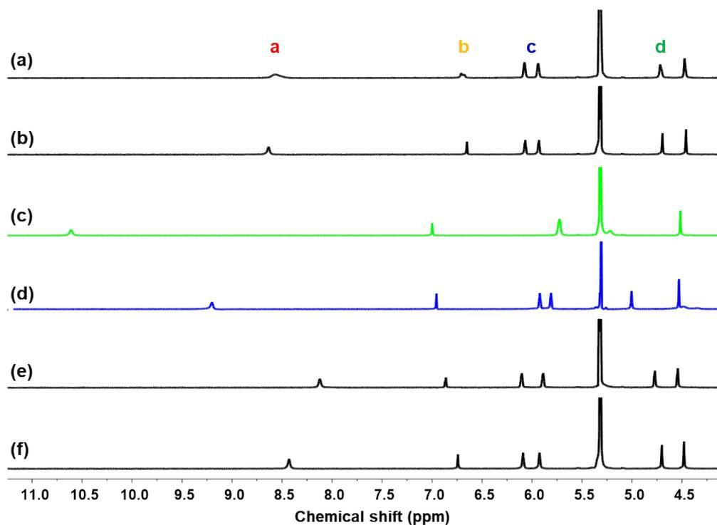
**Figure S1.** Partial  $^1\text{H}$  NMR spectra of (a) **1** and **1** with excess of (b) LiF(s), (c) LiCl(s), (d) LiBr(s), (e) LiI(s), and (f) LiClO<sub>4</sub>(s) (400 MHz, CD<sub>2</sub>Cl<sub>2</sub>:CD<sub>3</sub>OD=9:1, 297 K).
