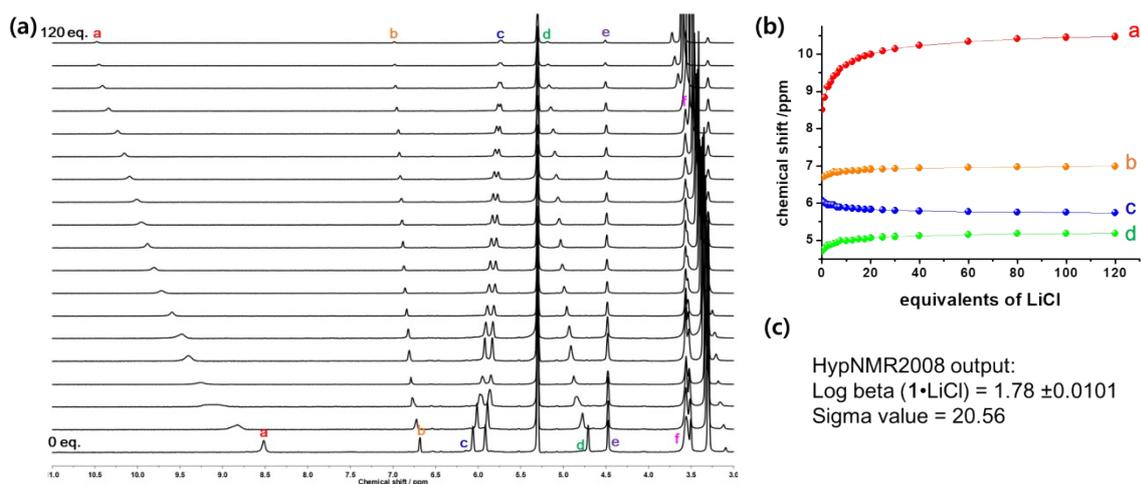
**Figure S4.** (a) stacked partial  $^1\text{H}$  NMR spectra of **1** (10 mM) with LiCl in 10%  $\text{CD}_3\text{OD}/\text{CD}_2\text{Cl}_2$ , (b) chemical shift changes of **1**'s protons upon addition of LiCl, (c) binding constant of **1**• LiCl calculated by HypNMR2008.
