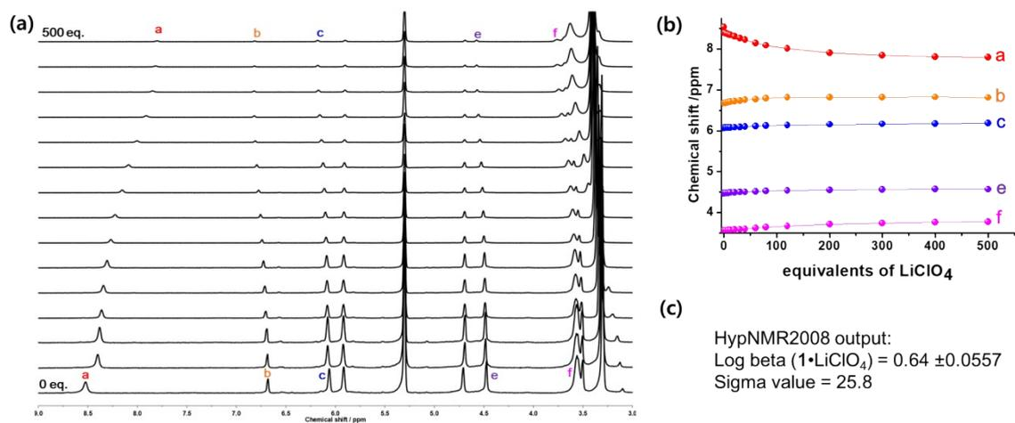
**Figure S6.** (a) stacked partial <sup>1</sup>H NMR spectra of **1** (10 mM) with LiClO<sub>4</sub> in 10% CD<sub>3</sub>OD/CD<sub>2</sub>Cl<sub>2</sub>, (b) chemical shift changes of **1**'s protons upon addition of LiClO<sub>4</sub>, (c) binding constant of **1**•LiClO<sub>4</sub> calculated by HypNMR2008.
