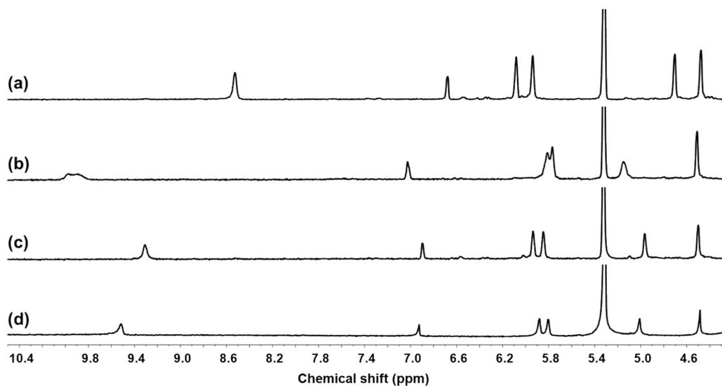
**Figure S3.** Partial  $^1\text{H}$  NMR spectra to confirm complexation of  $\mathbf{1}\cdot\text{LiBr}$  in solution state. (a) only  $\mathbf{1}$  and  $\mathbf{1}$  with (b) excess of TBABr, (c) TBABr followed by excess of  $\text{LiClO}_4$ , (d) excess of LiBr. (all spectra were recorded in 10%  $\text{CD}_3\text{OD}/\text{CD}_2\text{Cl}_2$ , 297 K)
