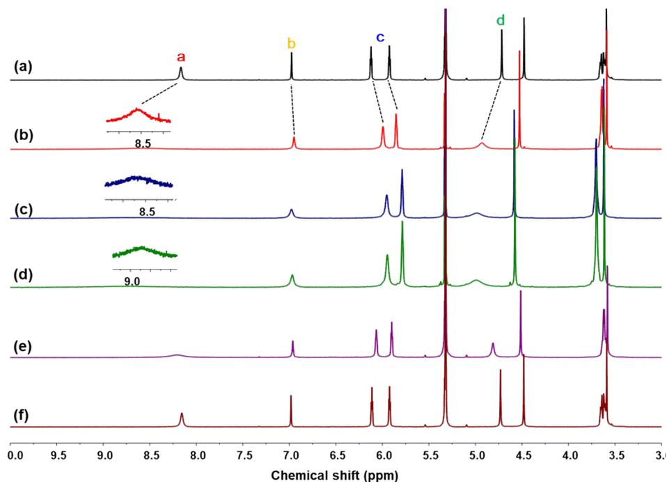
**Figure S13.**  $^1\text{H}$  NMR spectra of (a) **1** (5 mM) and **1** after extraction with (b) saturated LiBr(aq), (c) excess LiBr(s), (d) excess LiBr(s), NaBr(s) and KBr(s), (e) excess of NaBr (s), and (f) excess of KBr (s) (400 MHz,  $\text{CD}_2\text{Cl}_2$ , 297 K).
