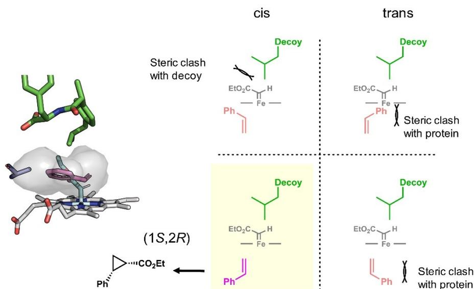
**Fig. S1** Proposed geometries of the reaction complex to allow cyclopropanation of styrene catalysed by the F87A/T268A mutant of P450BM3 in complex with R-Ibu-Phe. The least amount of steric repulsion is possible when styrene is in a conformation to yield the (1*S*,2*R*) isomer.
