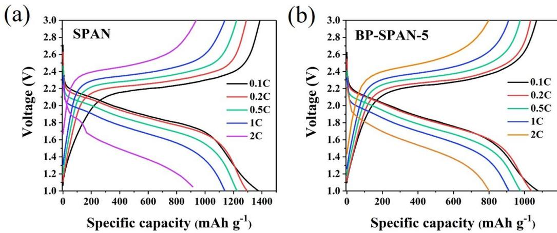
Fig. S7 (Dis-)Charge curves of cathodes at various C-rate, (a) SPAN, (b)BP-SPAN-5.
