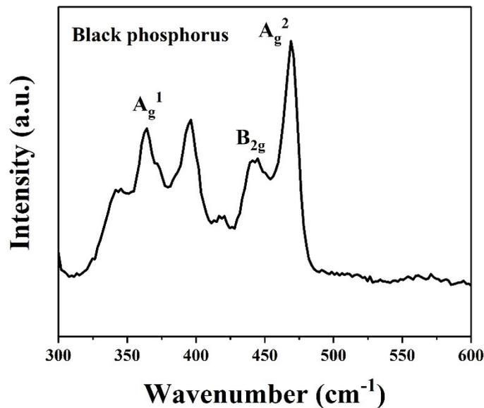
Fig. S1 Raman spectrum of black phosphorus.
