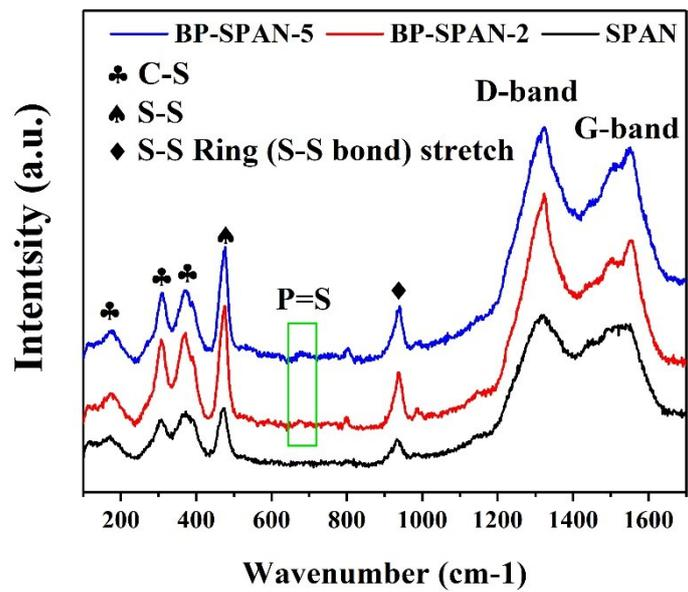
Fig. S3 Raman spectrum of SPAN, BP-SPAN-2 and BP-SPAN-5.
