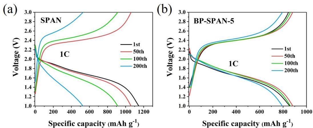
Fig. S8 Discharge/charge curves of cathodes for long cycling at 1C, (a) SPAN, (b)BP-SPAN-5.
