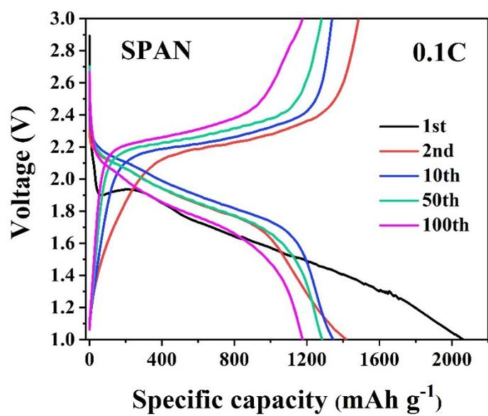
Fig. S4 (Dis-)Charge curves of SPAN at 0.1C.
