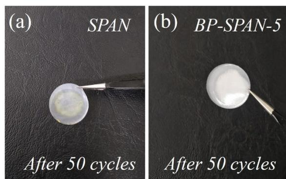
Fig. S5 The separator of disassembled cells after 50 cycles, (a) SPAN, (b) BP-SPAN-5.
