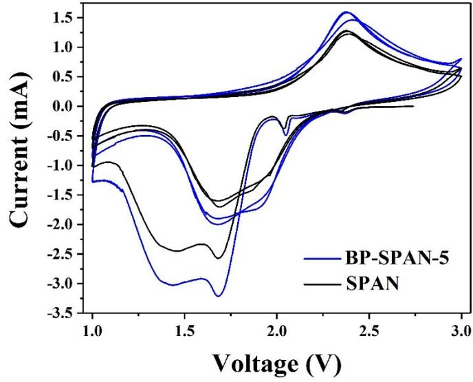
Fig. S6 CV curves of SPAN and BP-SPAN-5.
