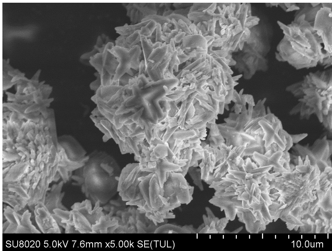
Fig. S1. FESEM image of Zn-N-C-1 microstars.
