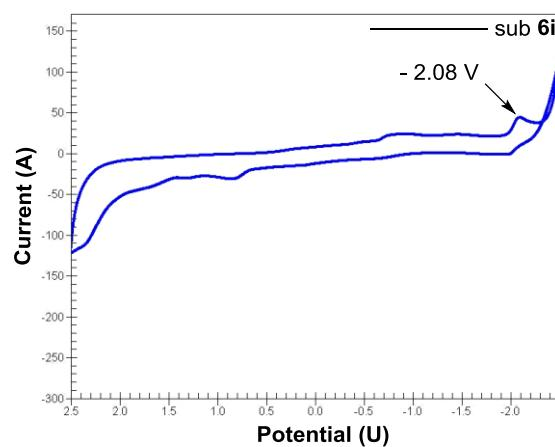
**Figure S3.** Cyclic voltammogram of substrate **6i**
