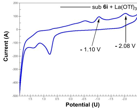
**Figure S4.** Cyclic voltammogram of substrate **6i**/La(OTf)<sub>3</sub> (1:1)
