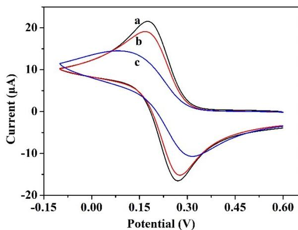
Figure S2. Cyclic voltammograms of DNA duplex modified gold electrode in 0.1 M KCl solution containing 5.0 mM  $K_3[Fe(CN)_6]$  at a scan rate of 100 mV/s. The data correspond to electrode before (a) and after modifications of 6-mercapto-1-hexanol (b), DNA/6-mercapto-1-hexanol (c), respectively.
