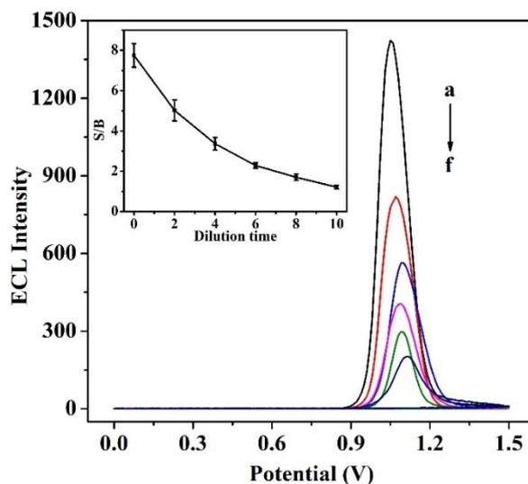
Figure S4. ECL response curves of gold electrodes modified in a mixture solution containing different ratios of duplex 1 and duplex 2. The dilution ratio of duplex 1 by duplex 2 is (a) no dilution, (b) 2, (c) 4, (d) 6, (e) 8, and (f) 10. Inset is a plot of the background-corrected ECL intensity as a function of the dilution ratio.
