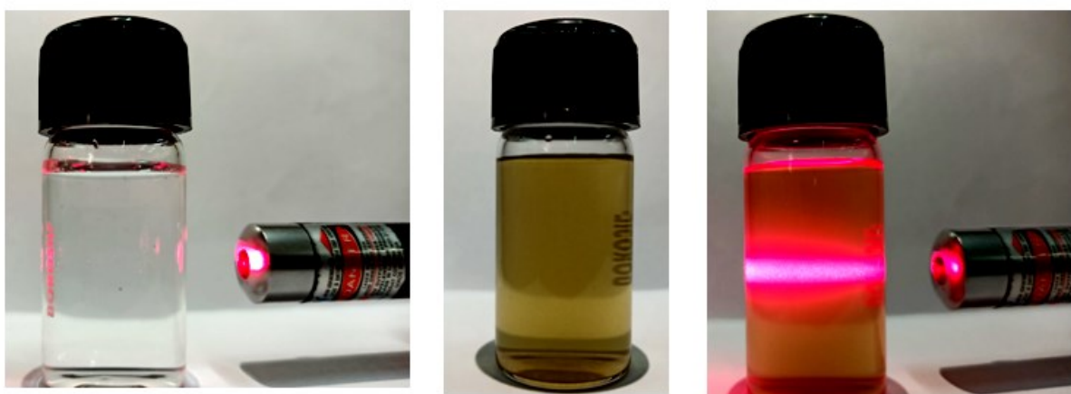
Figure S21. Photograph of Tyndall effect in presence of LASER beam. Blank water in presence of LASER light ( left ), aqueous solution of 2 ( middle ) and aqueous solution of 2 in presence of LASER light ( right ).
