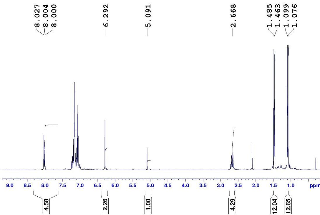
**Fig. S11**  $^1\text{H}$  NMR of 1:1 reation of **1a** with azobenzene in benzene- $\text{D}_6$  from crude reaction mixture at room temperature.
