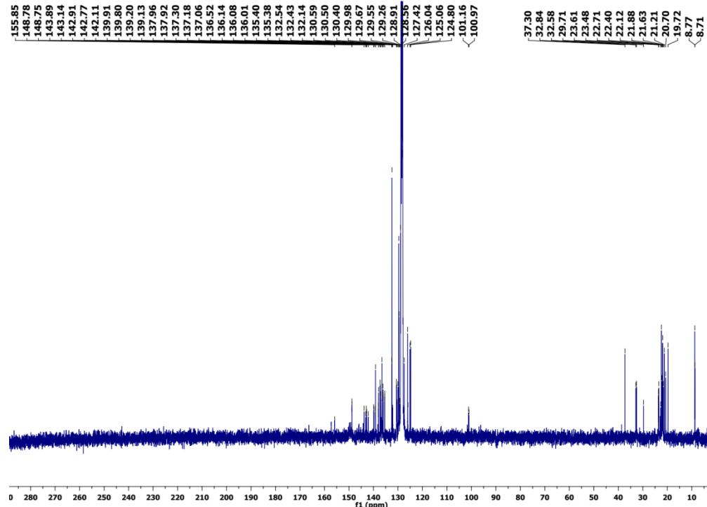
**Fig. S14**  $^{13}\text{C}\{^1\text{H}\}$  NMR spectrum of **6** in benzene-D<sub>6</sub> at room temperature.
