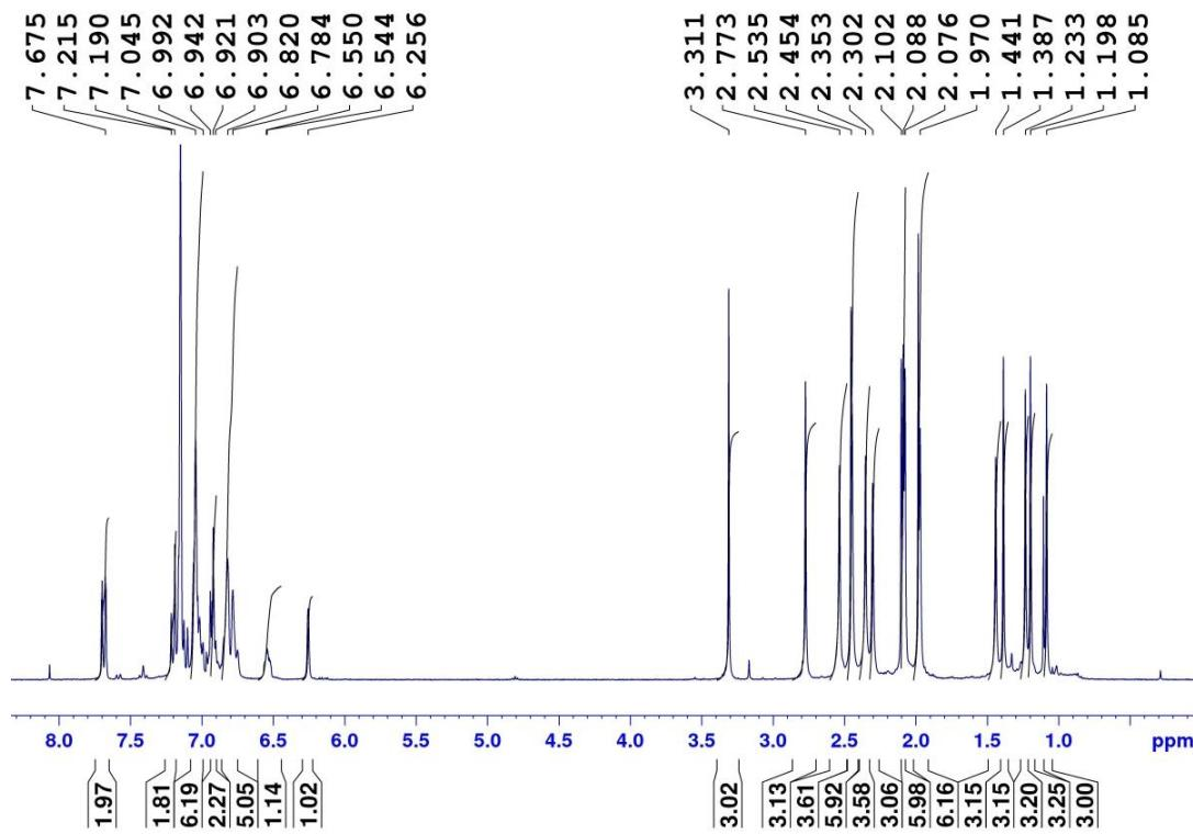
**Fig. S5** <sup>1</sup>H NMR spectrum of **6** in benzene-D<sub>6</sub> at room temperature.
