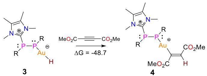
**Scheme S1** Relative energy for the reaction of **3** with dimethyl acetylenedicarboxylate at the M06-2X-D3/6-31G(d,p)(SDD)//B3LYP-D3/6-31G(d,p)(LANL2DZ) level of theory.
