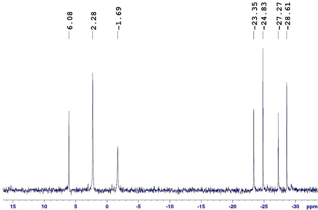
**Fig. S8** <sup>31</sup>P NMR spectrum from the crude reaction mixture of **3** and phenyl acetylene when the reaction was carried out at room temperature in benzene-D<sub>6</sub> at room temperature.
