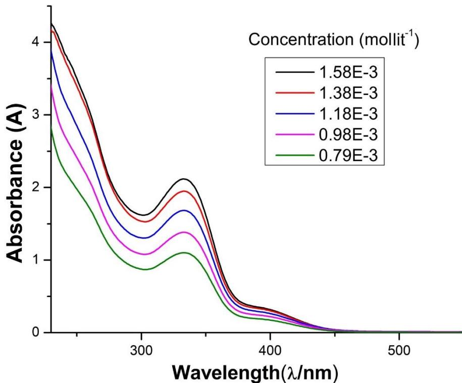
**Fig. S23** UV/Vis spectra of **5** in THF at room temperature.
