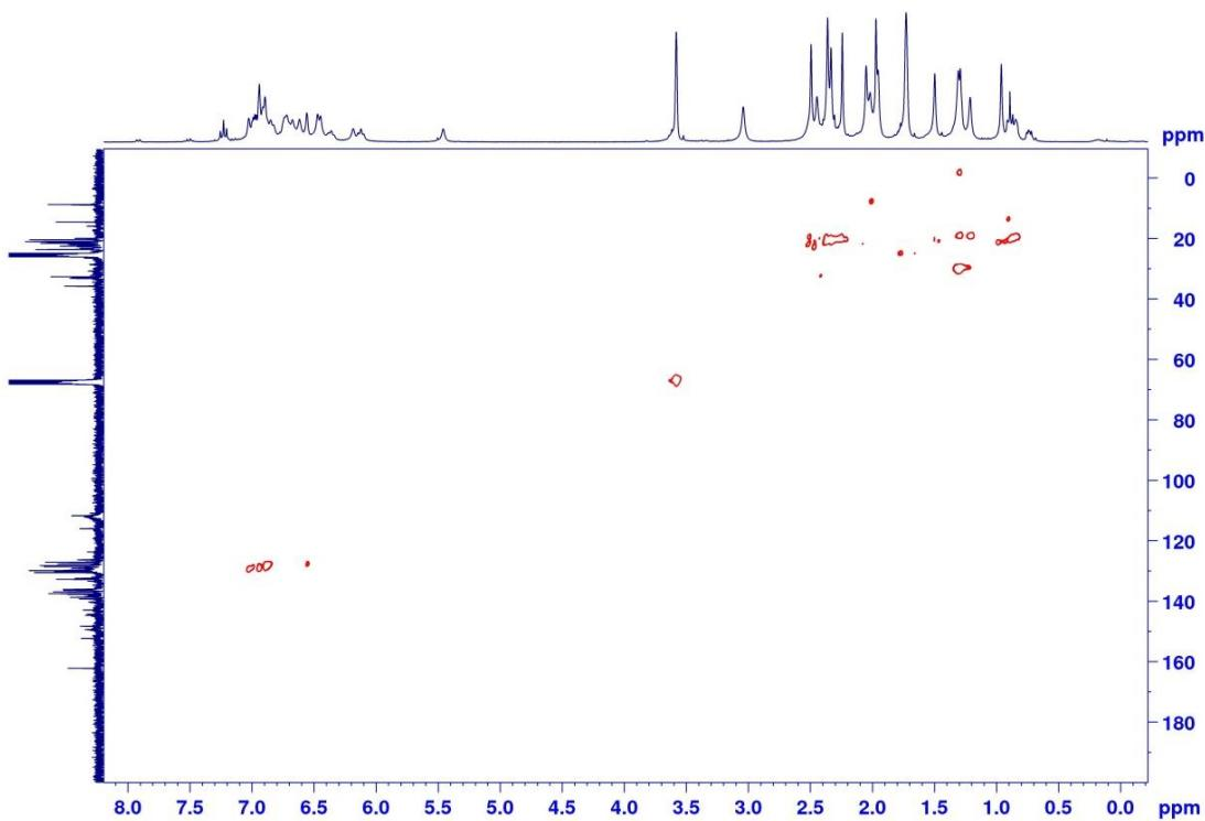
**Fig 19**  $^1\text{H}$ - $^{13}\text{C}\{^1\text{H}\}$  HSQC NMR spectrum of **7** in  $\text{THF}-\text{D}_8$  at room temperature.
