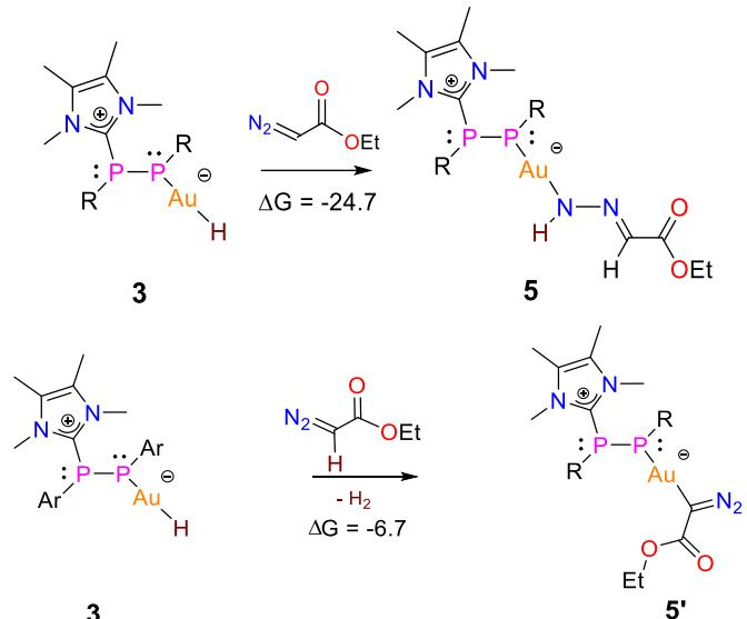
**Scheme S2** Relative energy for the reactions of **3** with ethyl diazoacetate at the M06-2X-D3/6-31G(d,p)(SDD)//B3LYP-D3/6-31G(d,p)(LANL2DZ) level of theory.
