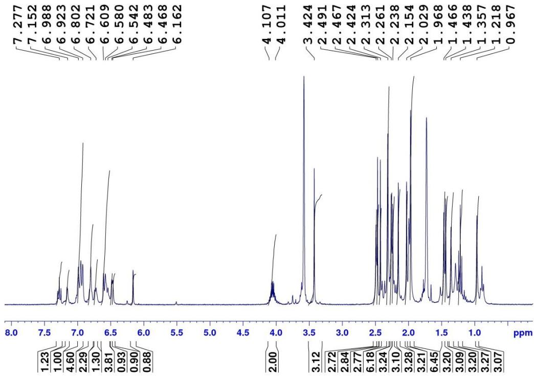
**Fig. S3**  $^1\text{H}$  NMR spectrum of **5** in  $\text{THF}-\text{D}_8$  at room temperature.
