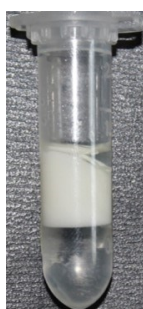
Fig. S3. Photographs of Pickering emulsions stabilized by both ZPs and SNCs after centrifugation at 20000 g for 30 min. The concentration of two different particles was fixed to 2 wt%, the pH of the aqueous phase was about 4 and oil-water volume ratio was fixed to 1:1. All emulsions were homogenized at 17000 rpm for 2 min.
