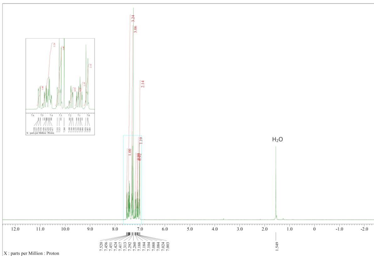
**Figure S41.**  $^1\text{H}$  NMR (400 MHz) spectrum of **3i** in  $\text{CDCl}_3$ .
