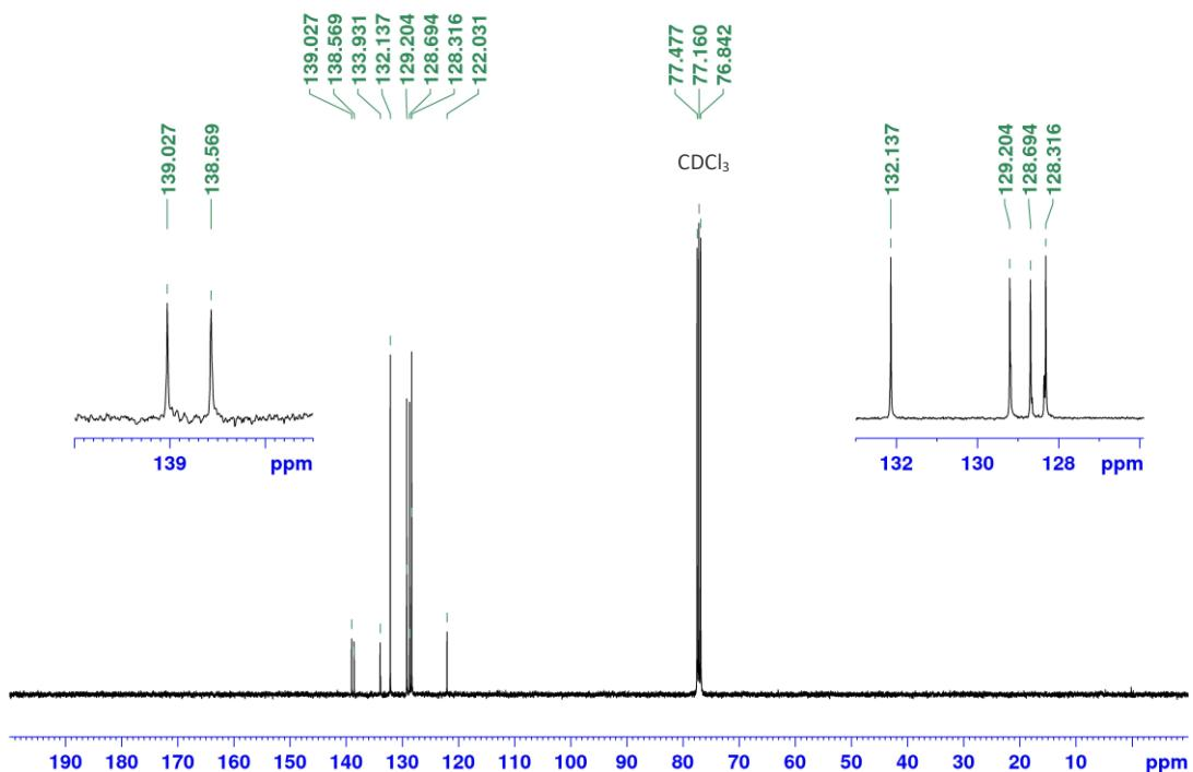
**Figure S30.**  $^{13}\text{C}$  NMR (100 MHz) spectrum of **3c** in  $\text{CDCl}_3$ .
