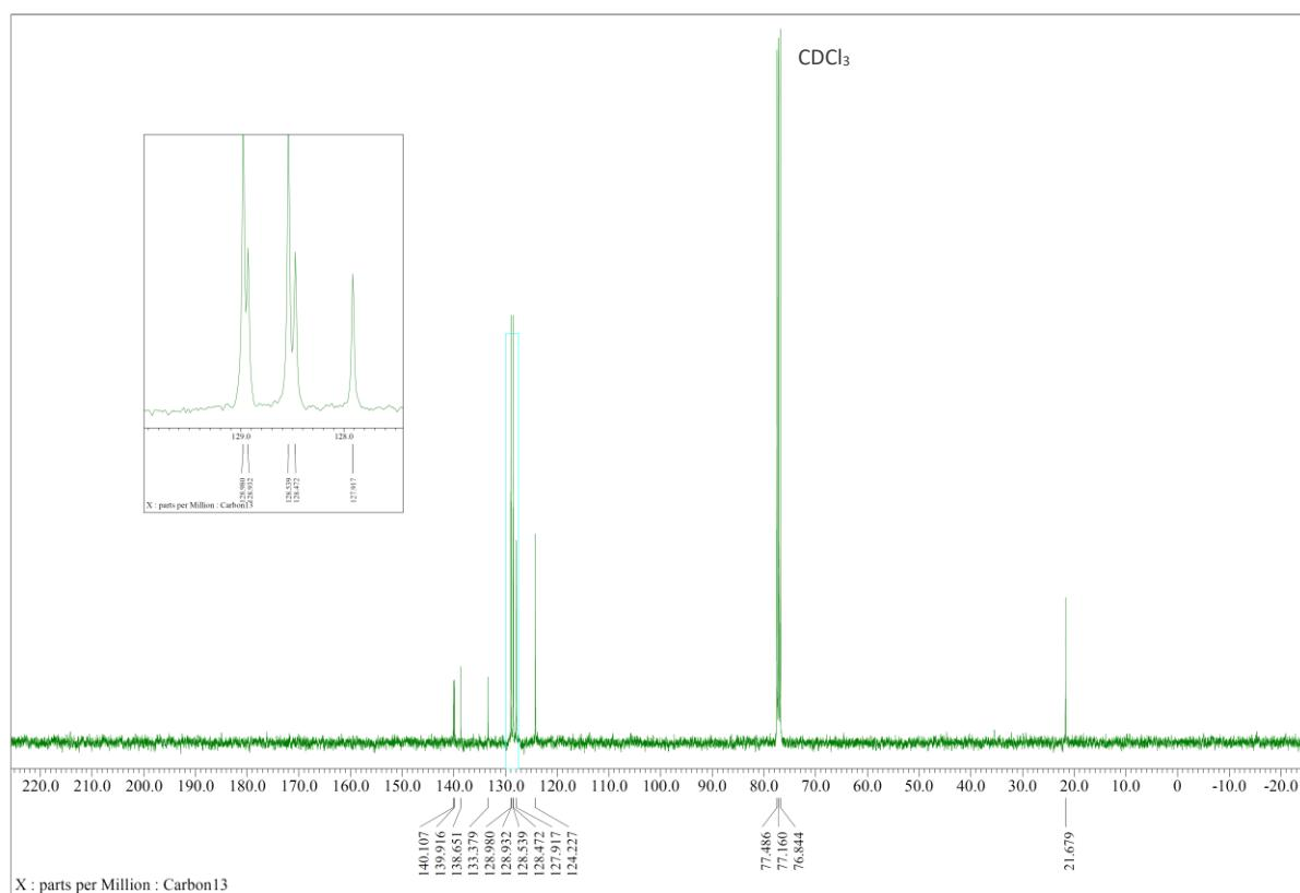
**Figure S68.** <sup>13</sup>C NMR (100 MHz) spectrum of **3v** in CDCl<sub>3</sub>.
