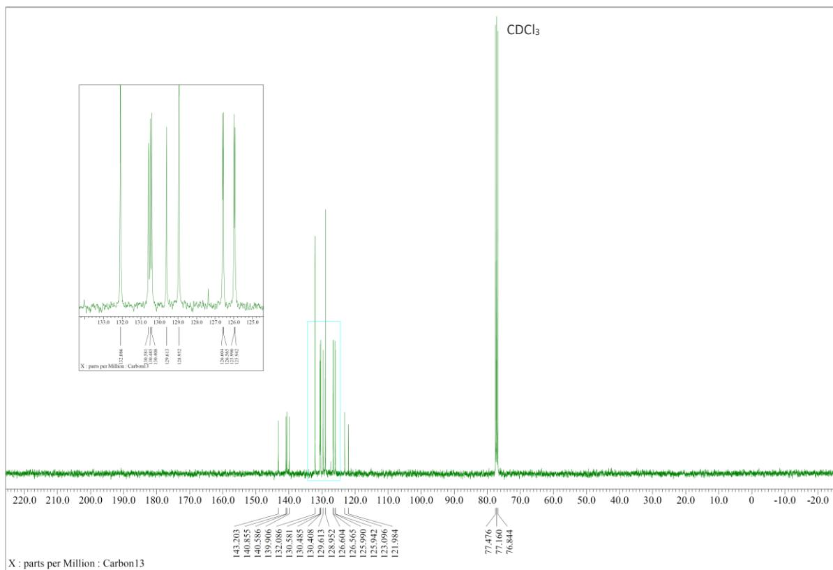
**Figure S40.** <sup>13</sup>C NMR (100 MHz) spectrum of **3h** in CDCl<sub>3</sub>.
