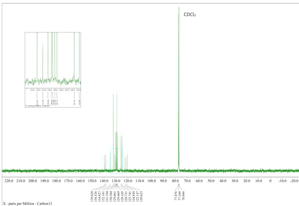
**Figure S44.** <sup>13</sup>C NMR (100 MHz) spectrum of **3j** in CDCl<sub>3</sub>.
