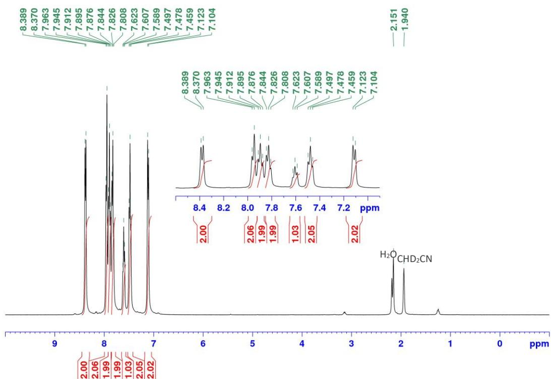
**Figure S9.** <sup>1</sup>H NMR (400 MHz) spectrum of **8** in  $\text{CD}_3\text{CN}$ .
