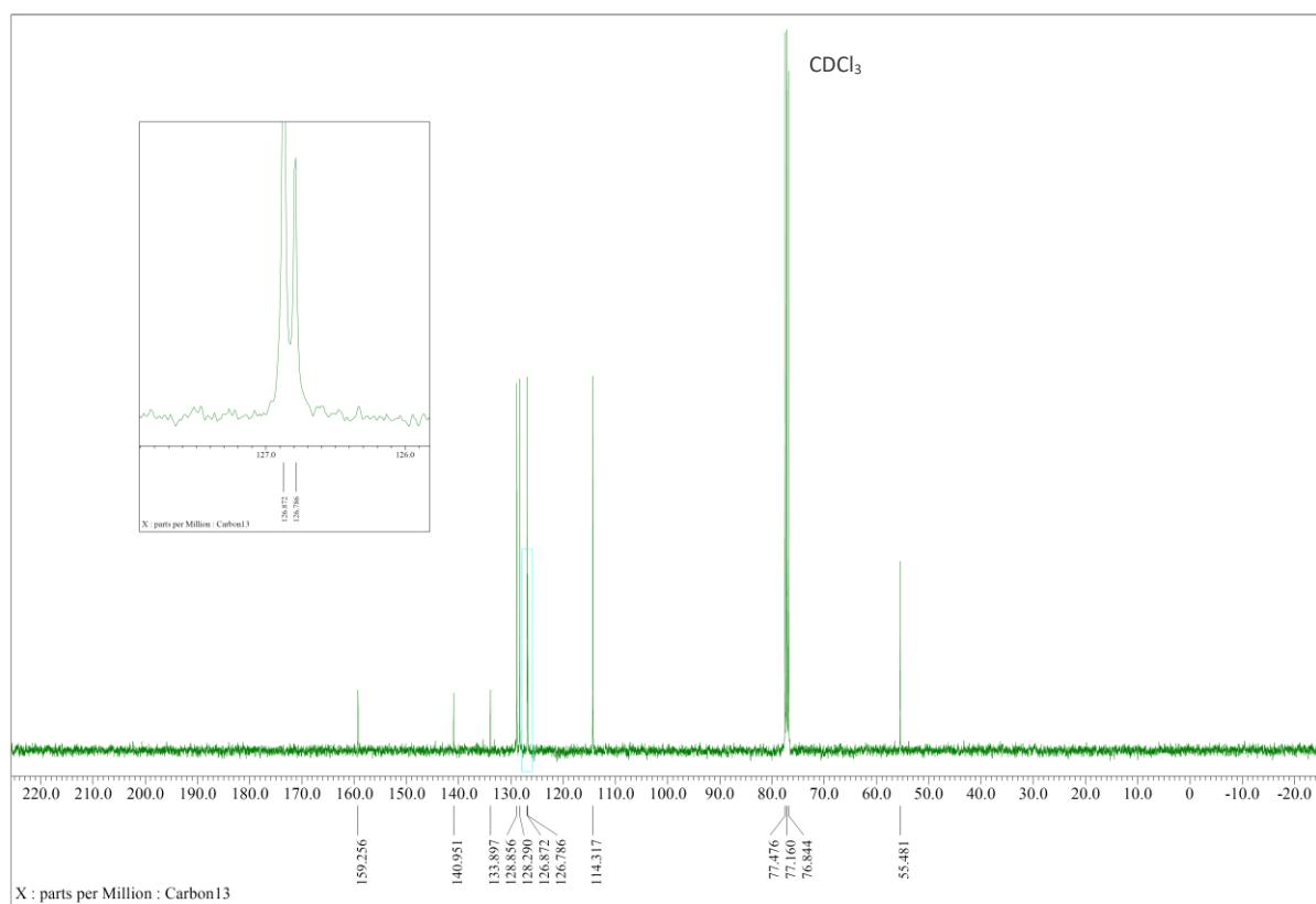
**Figure S62.**  $^{13}\text{C}$  NMR (100 MHz) spectrum of **3s** in  $\text{CDCl}_3$ .
