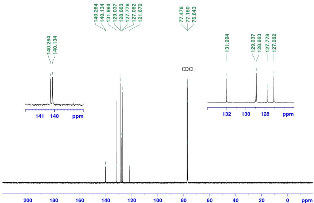
**Figure S28.**  $^{13}\text{C}$  NMR (100 MHz) spectrum of **3b** in  $\text{CDCl}_3$ .
