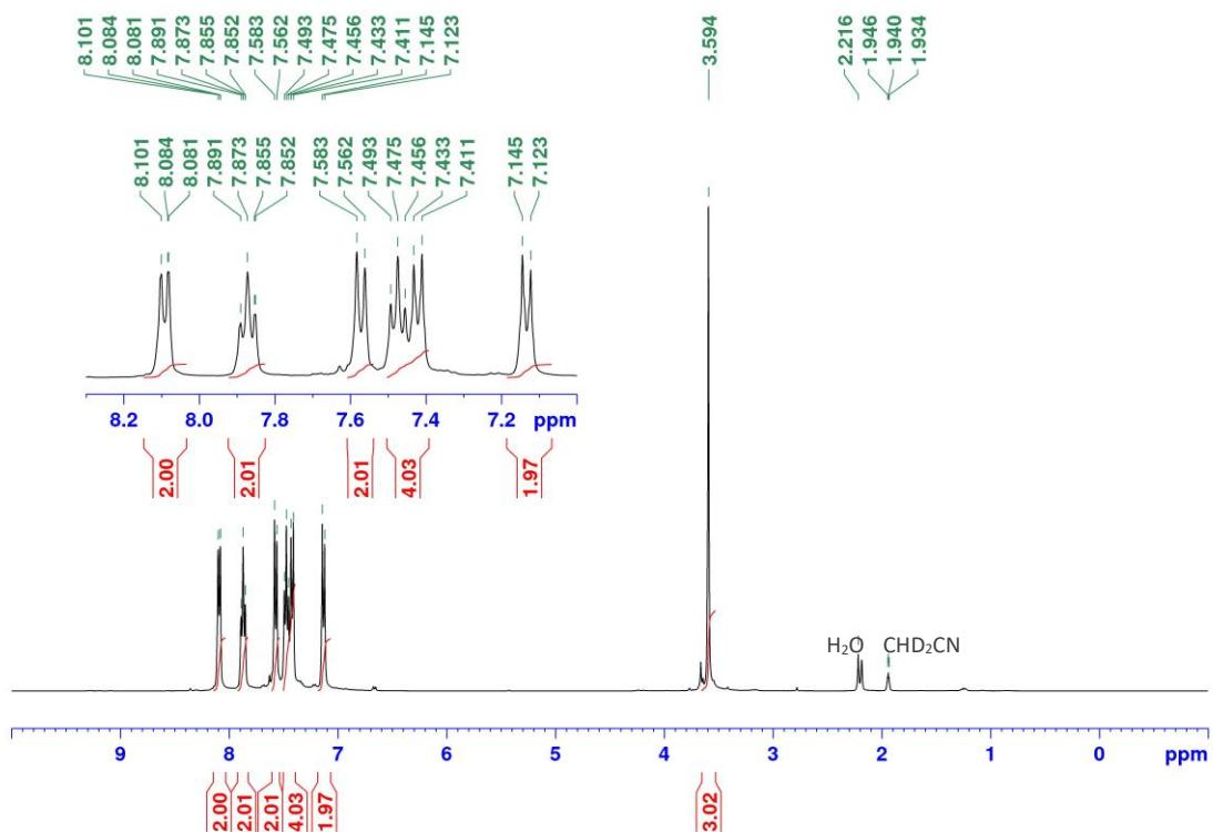
**Figure S11.** <sup>1</sup>H NMR (400 MHz) spectrum of **2b** in  $\text{CD}_3\text{CN}$ .
