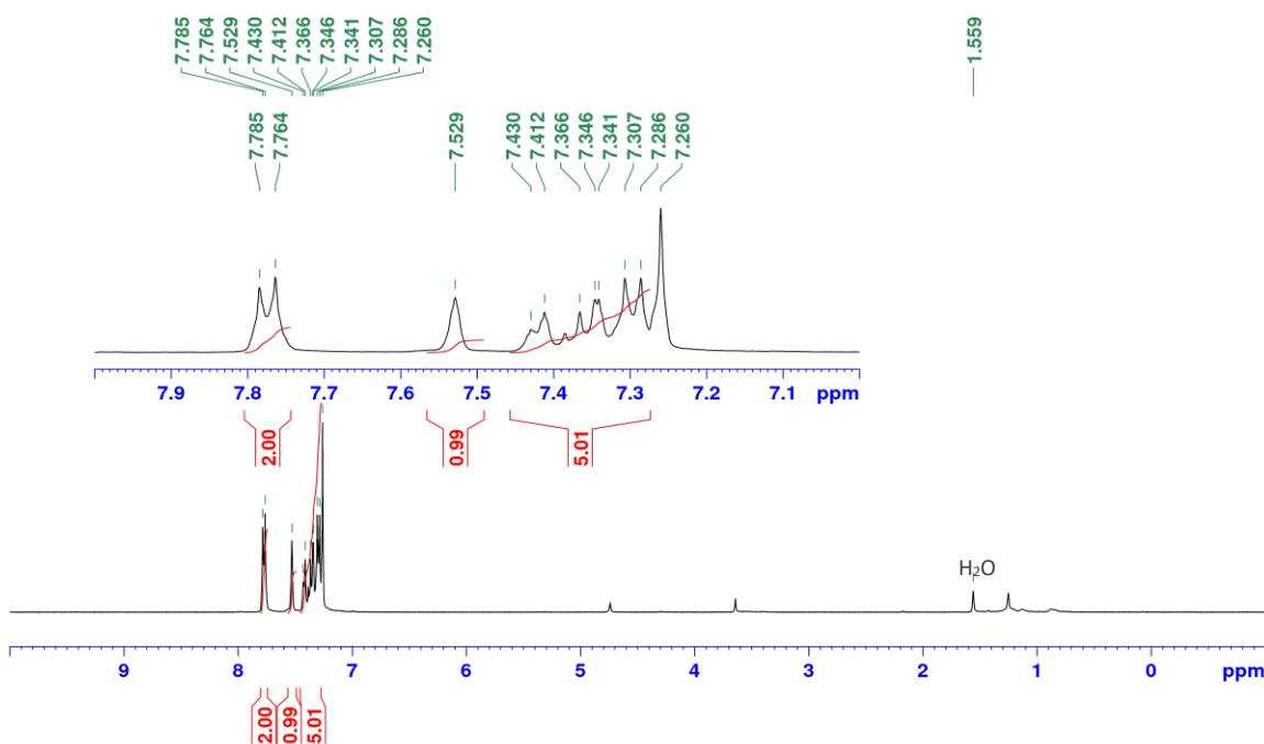
**Figure S51.** <sup>1</sup>H NMR (400 MHz) spectrum of **3n** in CDCl<sub>3</sub>.
