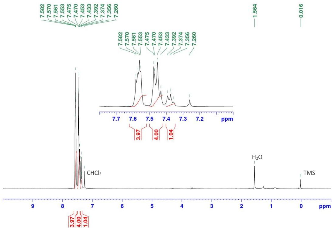
**Figure S27.** <sup>1</sup>H NMR (400 MHz) spectrum of **3b** in  $\text{CDCl}_3$ .
