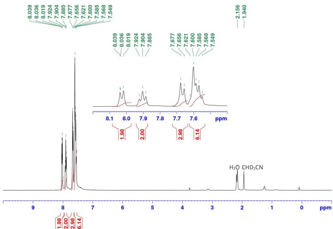
**Figure S7.**  $^1\text{H}$  NMR (400 MHz) spectrum of **5** in  $\text{CD}_3\text{CN}$ .
