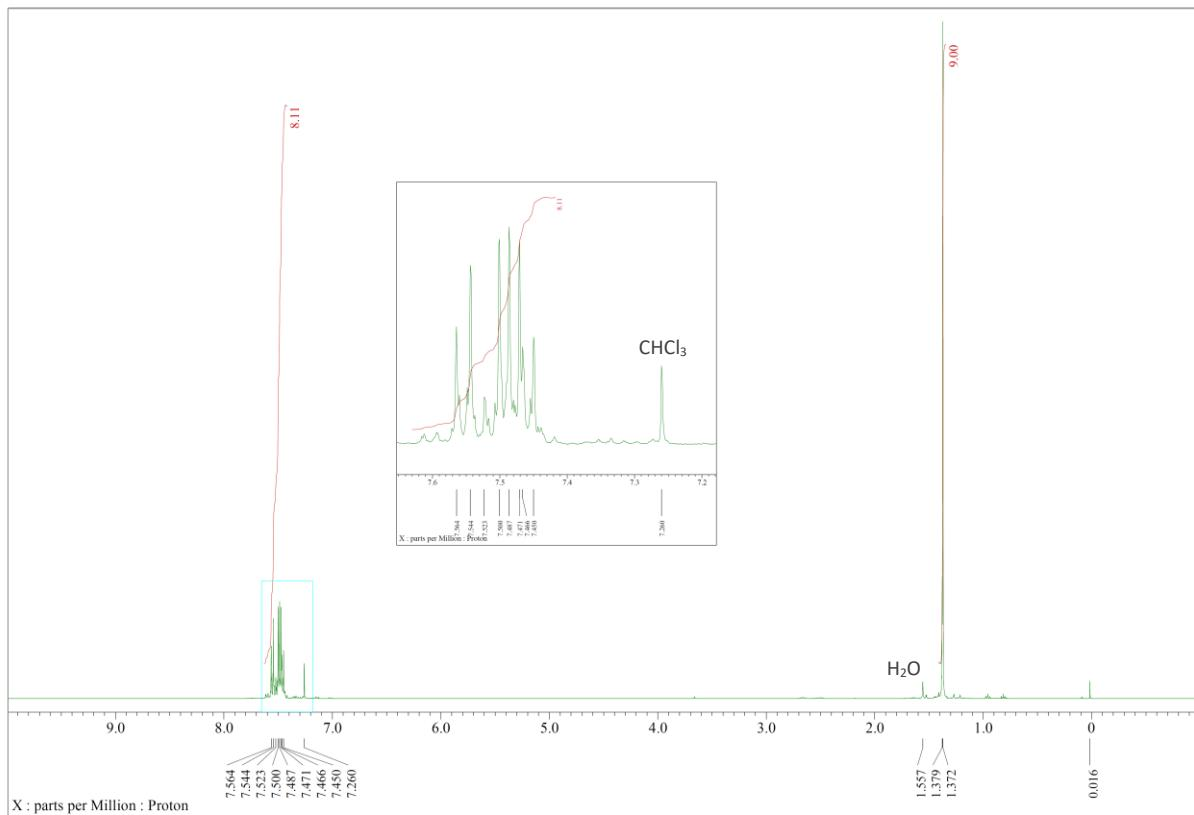
**Figure S31.** <sup>1</sup>H NMR (400 MHz) spectrum of **3d** in  $\text{CDCl}_3$ .
