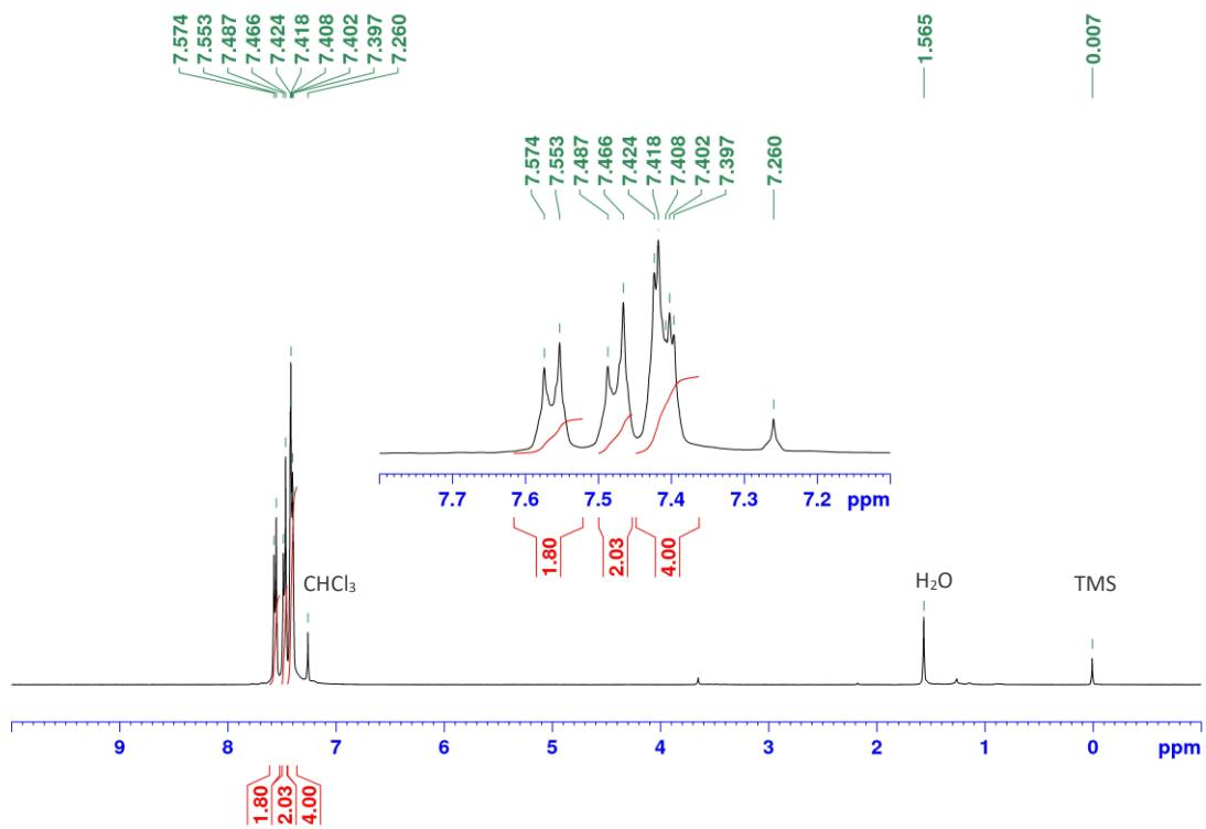
**Figure S29.** <sup>1</sup>H NMR (400 MHz) spectrum of **3c** in  $\text{CDCl}_3$ .
