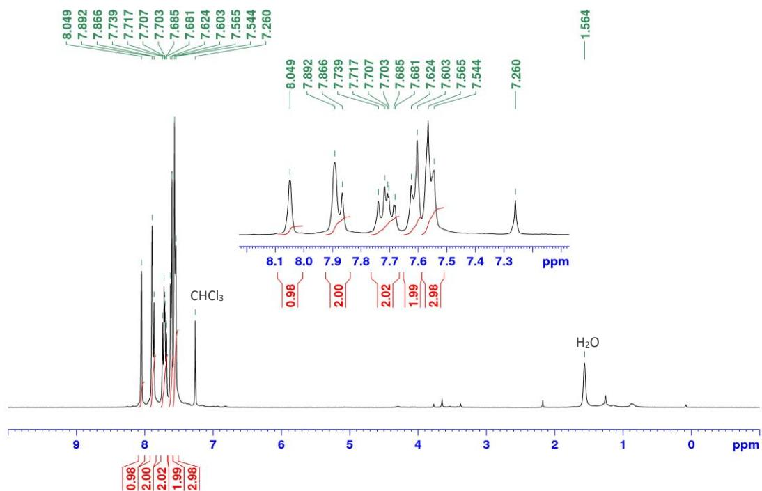
**Figure S43.** <sup>1</sup>H NMR (400 MHz) spectrum of **3j** in  $\text{CDCl}_3$ .
