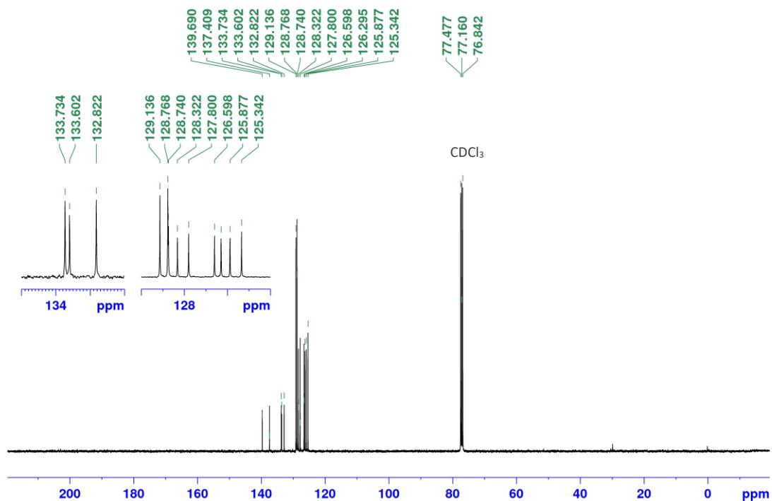
**Figure S72.**  $^{13}\text{C}$  NMR (100 MHz) spectrum of **3x** in  $\text{CDCl}_3$ .
