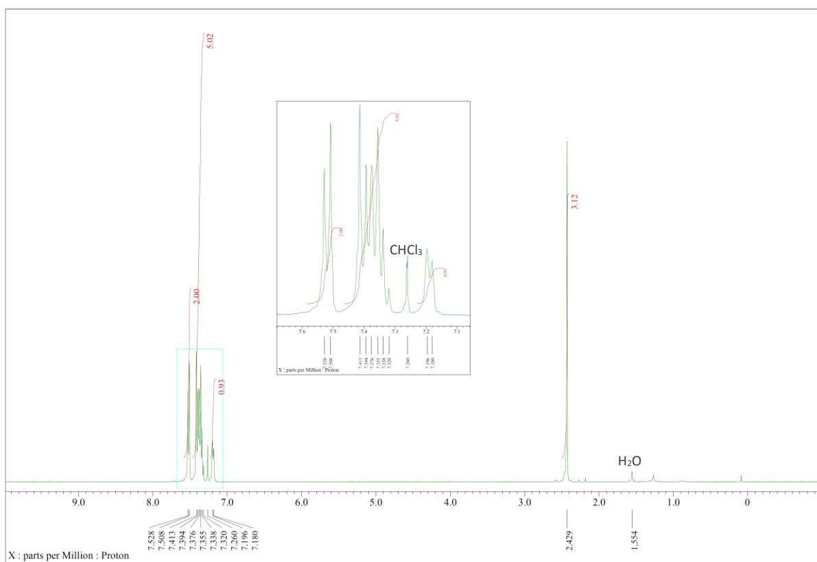
**Figure S67.** <sup>1</sup>H NMR (400 MHz) spectrum of **3v** in  $\text{CDCl}_3$ .
