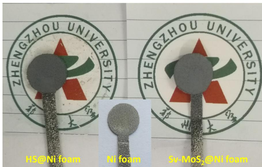
**Figure S7.** Photo of Sv-MoS<sub>2</sub> and amorphous MoO<sub>3-x</sub>/MoS<sub>2</sub> heterostructure (HS) loaded on Ni foam.
