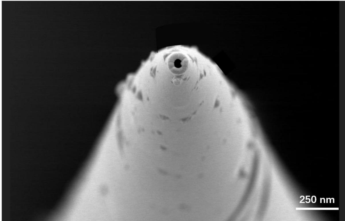
**Figure S1.** SEM image of the unmodified glass nanopore tip.
