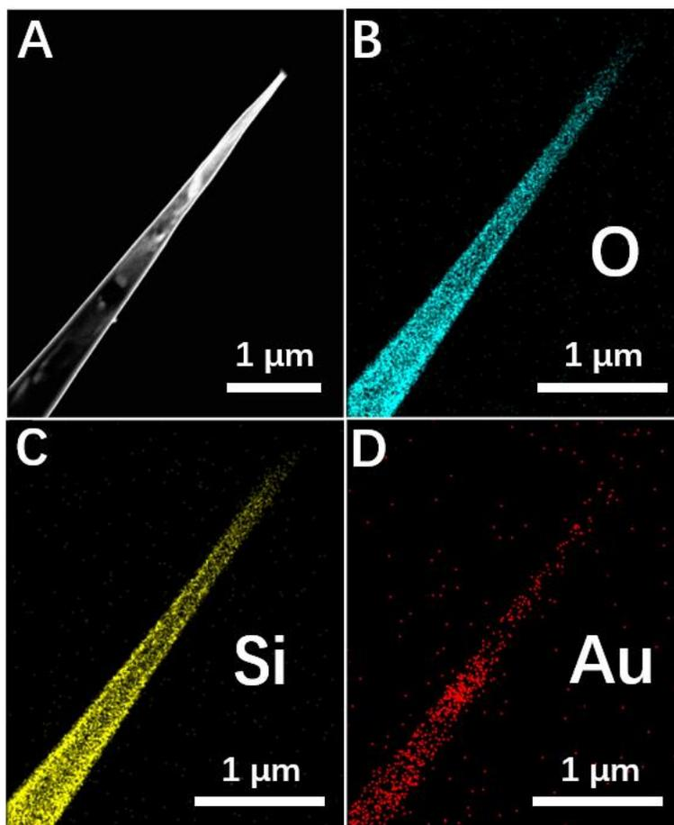
**Figure S4.** Dark-field TEM image (A) and the corresponding TEM elemental mappings (B-D, O, Si and Au) of Au membrane-coated glass nanopore.
