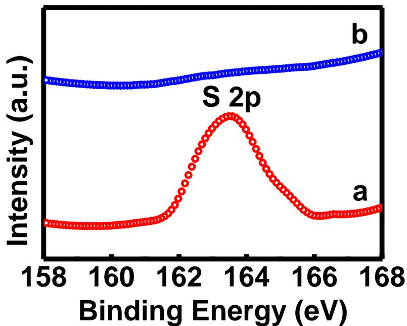
**Figure S5.** XPS for S 2p obtained at HAT-modified nanopipette electrode (a) before and (b) after treatment with 350 nM  $\bullet\text{OH}$ .
