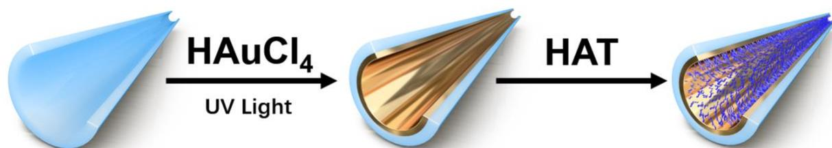
**Figure S2.** Stepwise modification of HAT functionalized nanopore.
