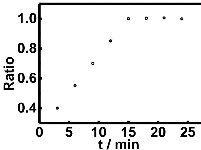
**Figure S6.** Effect of reaction time on ionic current change ratio at -1.0 V in the presence of Fenton reagent (350 nM  $\text{Fe}^{2+}$  + 2.1  $\mu\text{M}$   $\text{H}_2\text{O}_2$ ).
