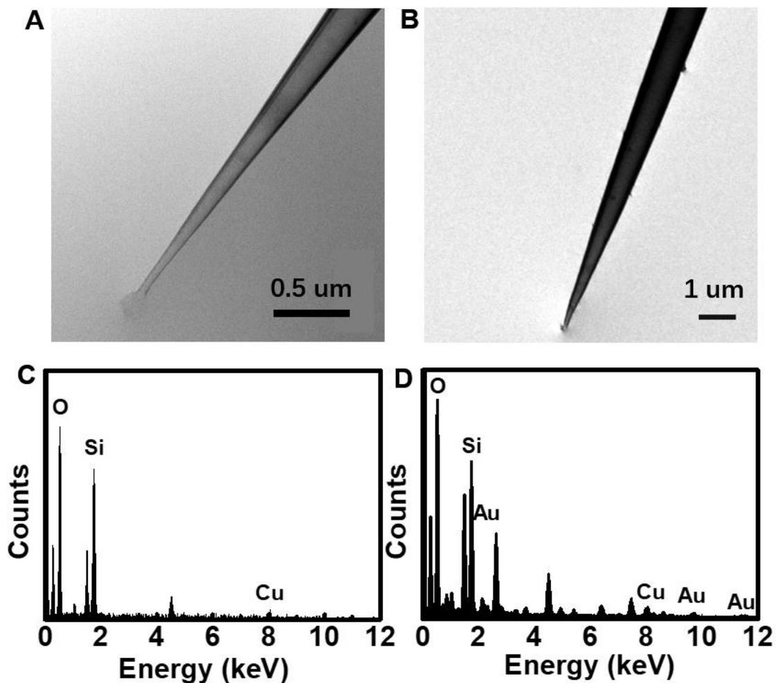
**Figure S3.** (A,B) medium-magnification TEM images and (C,D) EDX spectra of (A,C) the unmodified (Au-free) glass nanopore tip and (B,D) the Au-modified glass nanopore tip .
