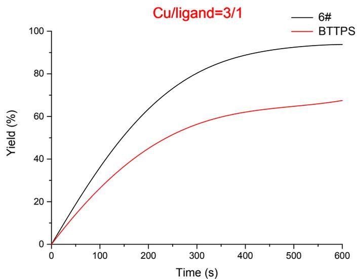
Figure S4. Catalytic performance of **6** and BTTPS at 3:1 Cu/**6** ratio. The reaction was carried out in PBS buffer (10 mM pH 7.4 PBS), 50  $\mu$ M prop-2-yn-1-ol and 100  $\mu$ M coumarin azide were added as substrates, 75  $\mu$ M CuSO<sub>4</sub> and 25  $\mu$ M ligand were added as catalyst, 2.5 mM sodium ascorbate was added as reducing reagent, and the reaction was carried out in air.
