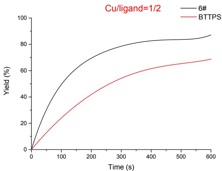
Figure S7. Catalytic performance of **6** and BTTPS at 1:2 Cu/**6** ratio. The reaction was carried out in PBS buffer (10 mM pH 7.4 PBS), 50  $\mu$ M prop-2-yn-1-ol and 100  $\mu$ M coumarin azide were added as substrates, 75  $\mu$ M CuSO<sub>4</sub> and 150  $\mu$ M ligand were added as catalyst, 2.5 mM sodium ascorbate was added as reducing reagent, and the reaction was carried out in air.
