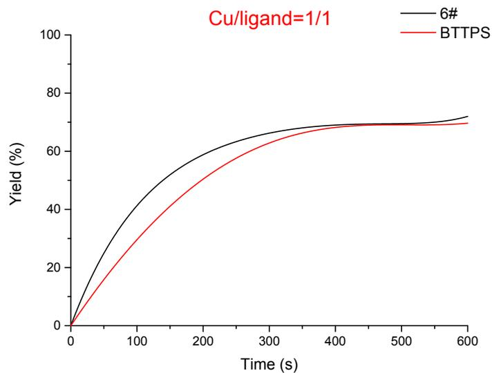
Figure S6. Catalytic performance of **6** and BTTPS at 1:1 Cu/**6** ratio. The reaction was carried out in PBS buffer (10 mM pH 7.4 PBS), 50  $\mu$ M prop-2-yn-1-ol and 100  $\mu$ M coumarin azide were added as substrates, 75  $\mu$ M CuSO<sub>4</sub> and 75  $\mu$ M ligand were added as catalyst, 2.5 mM sodium ascorbate was added as reducing reagent, and the reaction was carried out in air.
