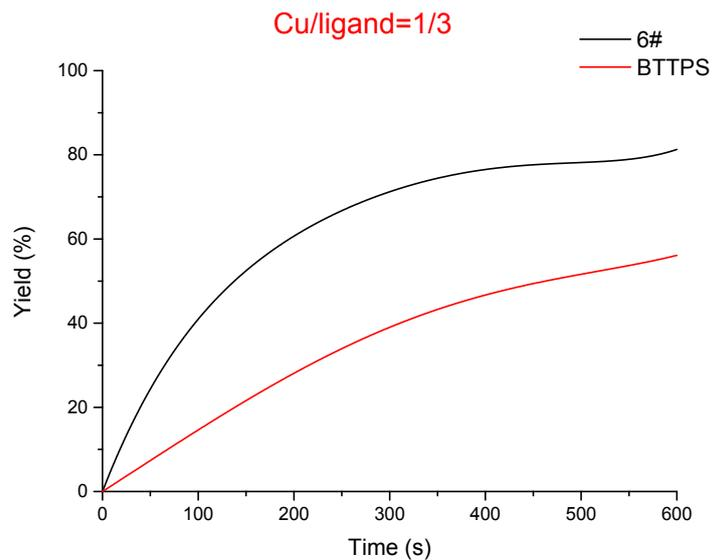
Figure 8. Catalytic performance of **6** and BTTPS at 1:3 Cu/**6** ratio. The reaction was carried out in PBS buffer (10 mM pH 7.4 PBS), 50  $\mu$ M prop-2-yn-1-ol and 100  $\mu$ M coumarin azide were added as substrates, 75  $\mu$ M CuSO<sub>4</sub> and 225  $\mu$ M ligand were added as catalyst, 2.5 mM sodium ascorbate was added as reducing reagent, and the reaction was carried out in air.
