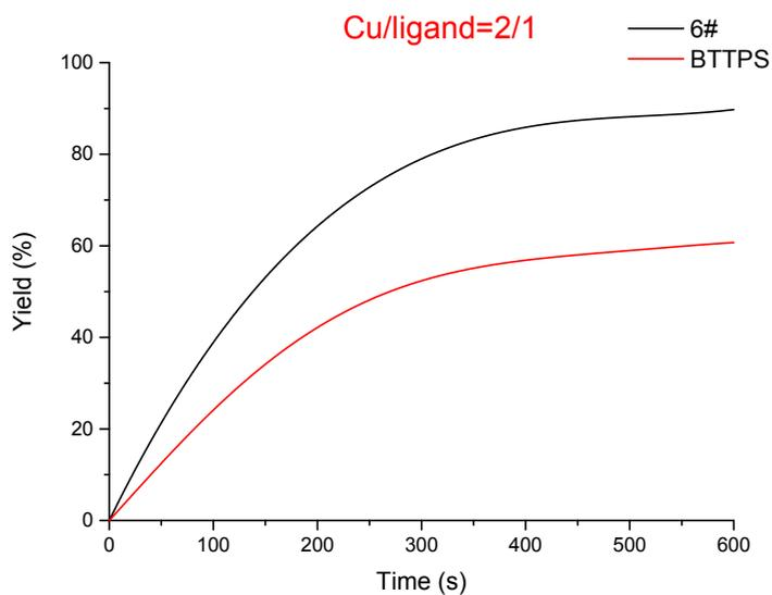
Figure S5. Catalytic performance of **6** and BTTPS at 2:1 Cu/**6** ratio. The reaction was carried out in PBS buffer (10 mM pH 7.4 PBS), 50  $\mu$ M prop-2-yn-1-ol and 100  $\mu$ M coumarin azide were added as substrates, 75  $\mu$ M CuSO<sub>4</sub> and 37.5  $\mu$ M ligand were added as catalyst, 2.5 mM sodium ascorbate was added as reducing reagent, and the reaction was carried out in air.
