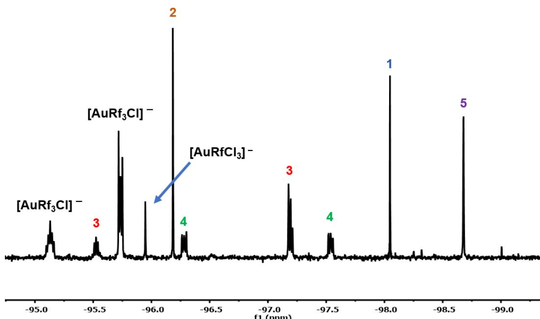
**Figure ESI2.** Expansion of the  $\text{F}_{\text{ortho}}$  region of the  $^{19}\text{F}$  NMR spectrum from the reaction aliquot (in  $\text{Et}_2\text{O}$ , ref. acetone- $d_6$ ) with signal assignment.
