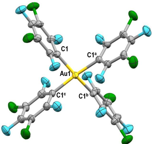
**Figure ESI7.** Molecular structure of  $[\text{AuRf}_4]^-$  (**8**).  $\text{NBu}_4^+$  is omitted for clarity. Selected bond lengths ( $\text{\AA}$ ) and angles ( $^\circ$ ):  $\text{Au}(1)\text{--C}(1) = 2.059(5)$ ;  $\text{C}(1)\text{--Au}(1)\text{--C}(1^a) = 90.46(3)$ ;  $\text{C}(1)\text{--Au}(1)\text{--C}(1^b) = 169.7(6)$ .
