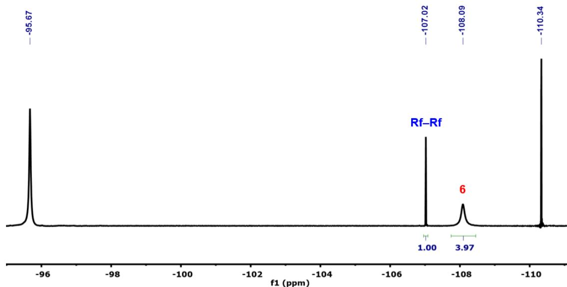
**Figure ESI3.** <sup>19</sup>F NMR spectrum recorded from a solution of **6** in CDCl<sub>3</sub> after 5 hours at 293 K with integrated F<sub>para</sub> signals.
