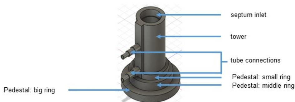
Figure 7: CAD-Design of Injection port for substrate and solvent.<sup>[6]</sup>
