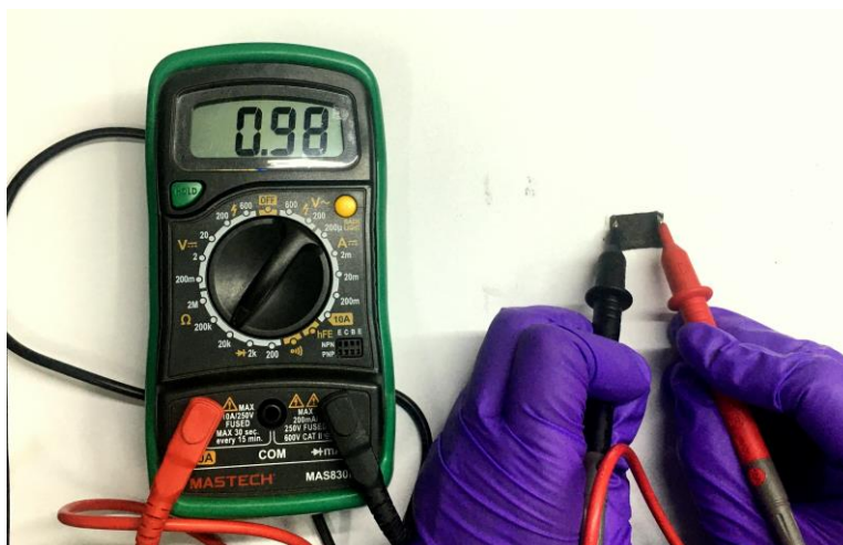
Fig. S7 Digital photograph of the electrical resistance measurement of the S@C fiber cloth by a digital multimeter.
