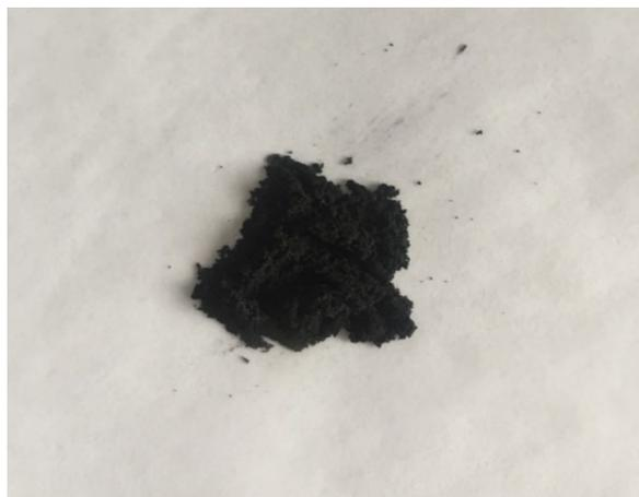
**Figure S1.** Digital image of as-prepared Fe<sub>2</sub>B nanoparticles.
