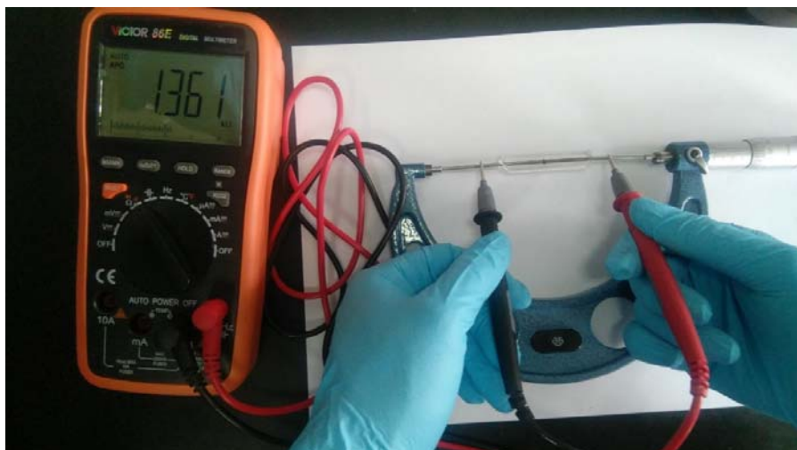
Fig. S40 A photograph of the setup for electronic conductivity measurement.
