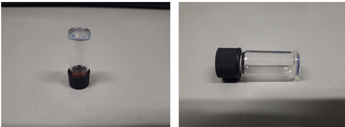
Figure S4. Photographs showing the gel formation at room temperature (20-22 °C) of the solution when the concentration of rac -BFA is increased to 18 mM in 1-phenyloctane.
