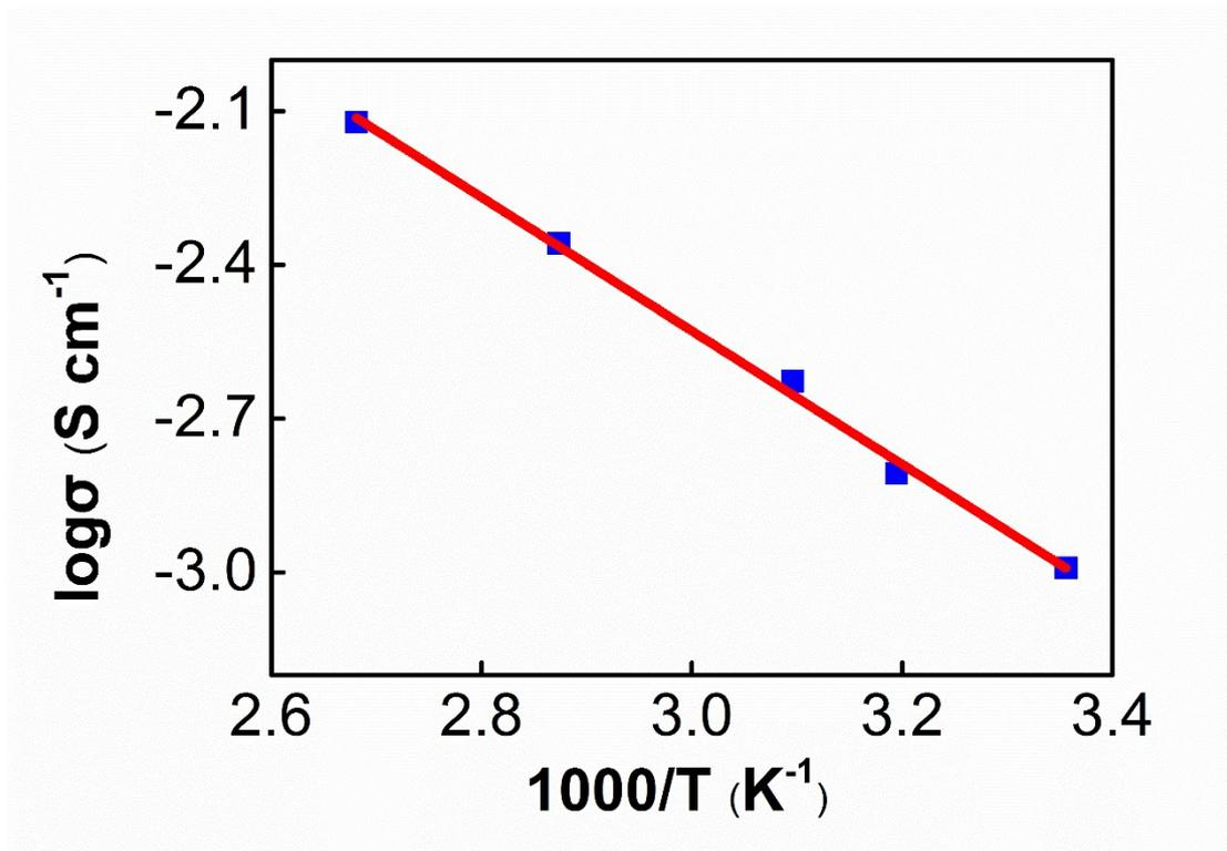
**Figure S3.** Arrhenius curve of the nano-grained  $\text{Na}_3\text{Zr}_2\text{Si}_2\text{PO}_{12}$ .
