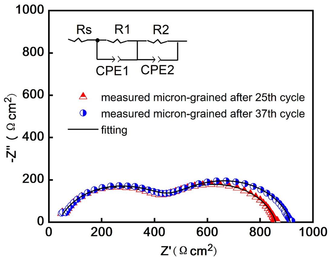
**Figure S5.** Nyquist plots of Na/micron-grained  $\text{Na}_3\text{Zr}_2\text{Si}_2\text{PO}_{12}/\text{Na}$  symmetrical cell for the 25<sup>th</sup> and 37<sup>th</sup> cycling.
