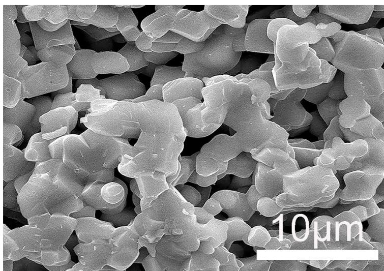
**Figure S2.** Top SEM view of controlled micron-grained  $\text{Na}_3\text{Zr}_2\text{Si}_2\text{PO}_{12}$  sintering at 1260 °C.
