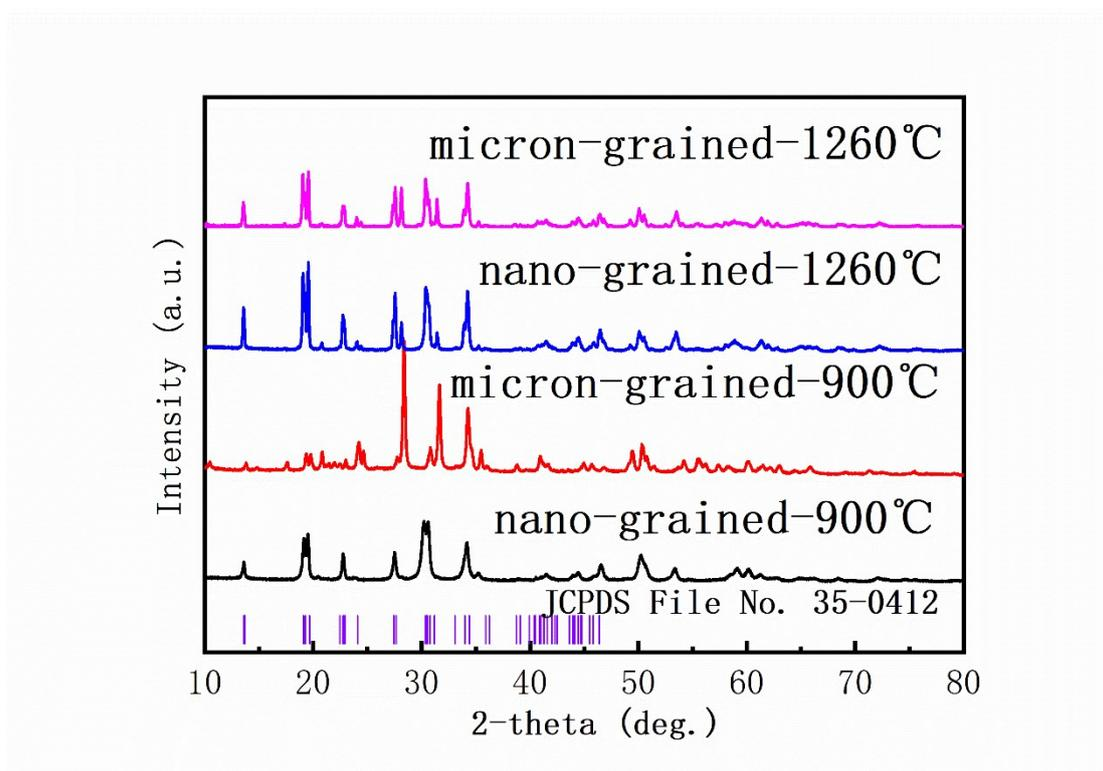
**Figure S1.** XRD patterns of the nano-grained and controlled micron-grained  $\text{Na}_3\text{Zr}_2\text{Si}_2\text{PO}_{12}$  annealing at 900 °C and sintering at 1260 °C.
