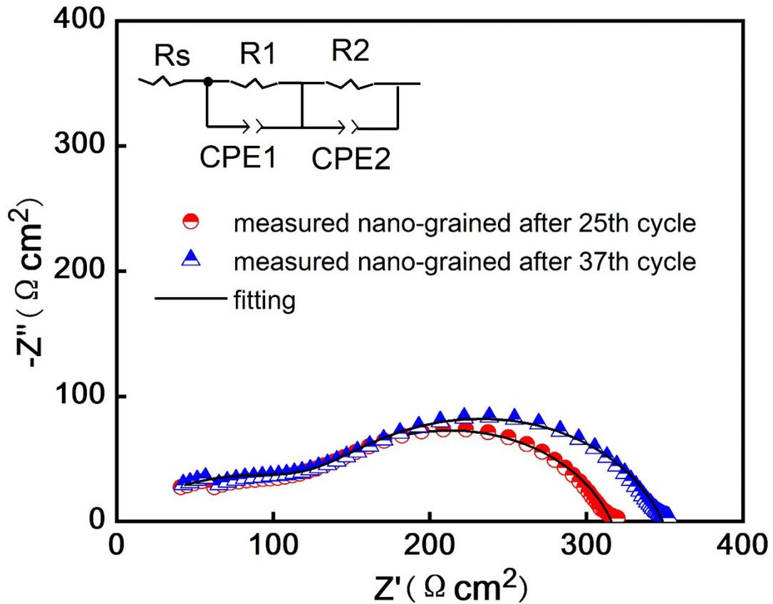
**Figure S4.** Nyquist plots of Na/nano-grained  $\text{Na}_3\text{Zr}_2\text{Si}_2\text{PO}_{12}/\text{Na}$  symmetrical cell for the 25<sup>th</sup> and 37<sup>th</sup> cycling. A  $(R_s)(R_1CPE_1)(R_2CPE_2)$  equivalent circuit (inset of Fig. 3d) is used to fit the impedance spectra, where  $R_s$  and  $R_1$  represent the grain and grain-boundary resistances of the electrolyte, and  $R_2$  represents the interfacial resistances for Na and electrolyte, CPE represents a constant phase element.
