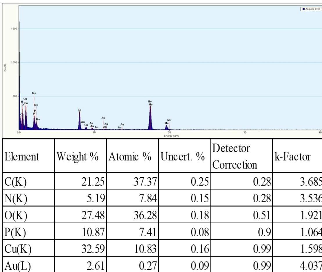
**Fig. S2** EDX pattern of the c-probe/AuNPs/Cu<sub>3</sub>(PO<sub>4</sub>)<sub>2</sub> HNFs.
