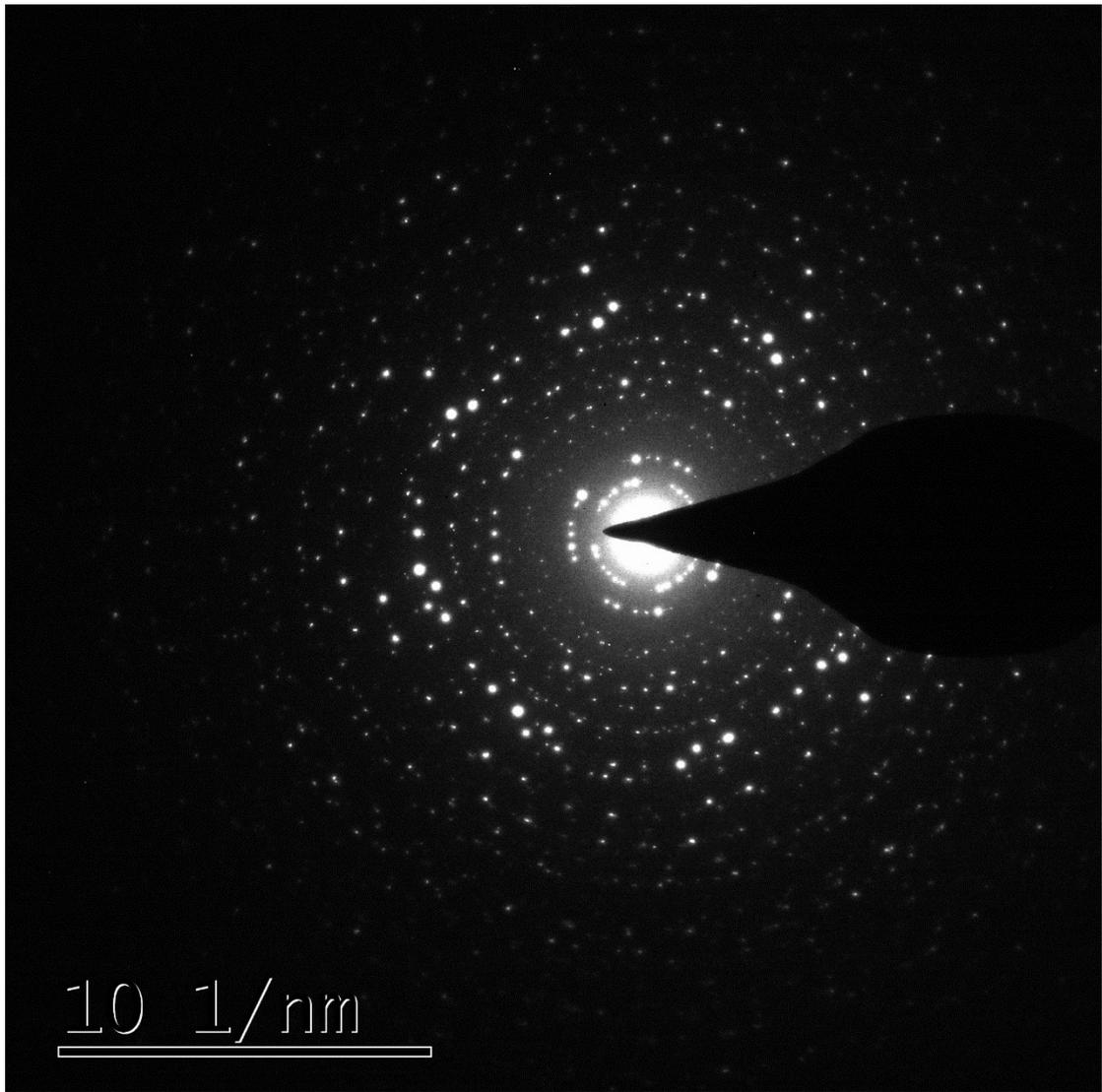
**Fig. S1** SAED pattern of the c-probe/AuNPs/Cu<sub>3</sub>(PO<sub>4</sub>)<sub>2</sub> HNFs.
