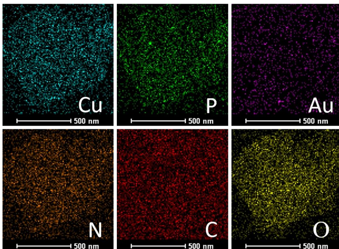
**Fig. S3** STEM-EDX mapping analyses of the c-probe/AuNPs/Cu<sub>3</sub>(PO<sub>4</sub>)<sub>2</sub> HNFs.
