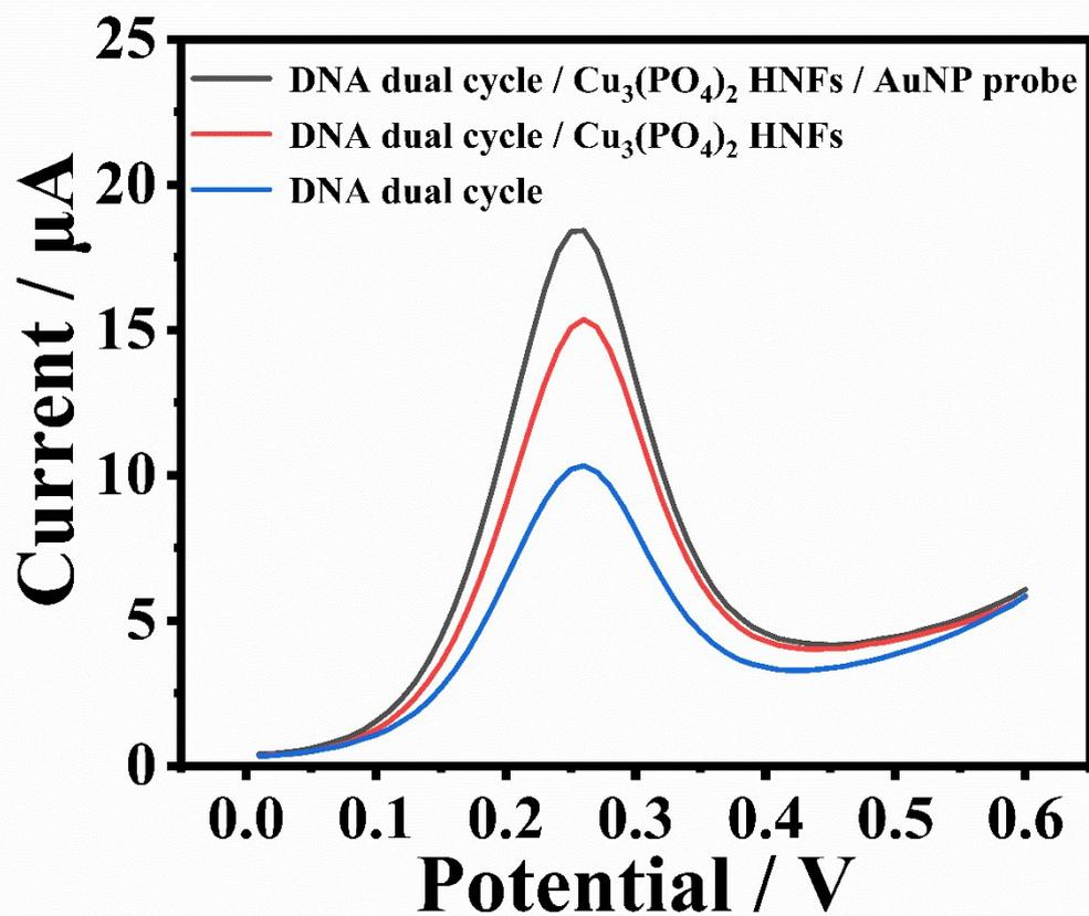
**Fig. S7** SWV response of different capture probes. The concentration of  $\text{Hg}^{2+}$  was 10.00 pM.
