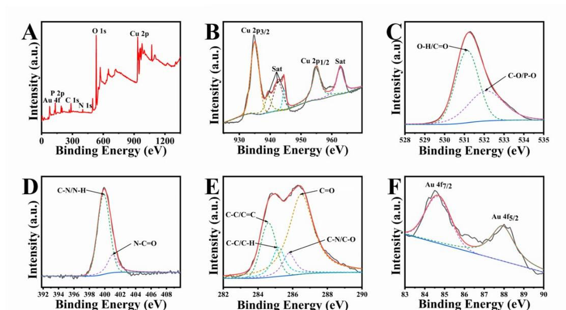
**Fig. S4** XPS survey spectra of c-probe/AuNPs/Cu<sub>3</sub>(PO<sub>4</sub>)<sub>2</sub> HNFs (A) survey spectrum, (B) C 1s, (C) Au 4f, (D) Cu 2p, (E) N 1s and (F) O 1s.
