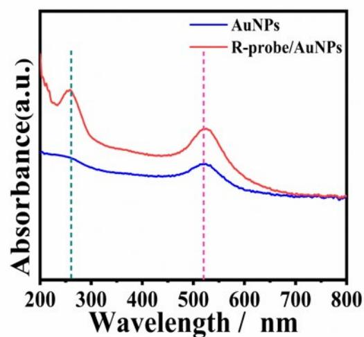
**Fig. S5** UV-vis absorbance spectrum of AuNPs and R-probe/AuNPs.
