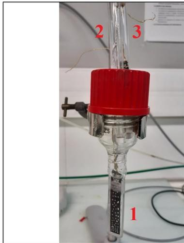
1. Carbon paper electrode with holes that allow the light to pass
