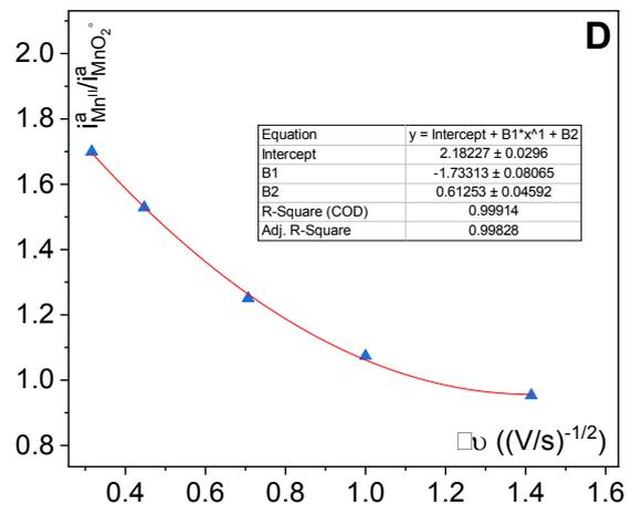
**Figure S1:** CVs of 0.5 mM Mn<sup>III</sup>(TPP)Cl on a 0.3 cm glassy carbon electrode, at 298 K, in 0.1 M TBAPF<sub>6</sub> / CH<sub>2</sub>Cl<sub>2</sub> solution at various scan rate (0.1, 0.2, 0.5, 1 and 2 V/s). **A)** Under Ar. **B)** Under O<sub>2</sub>. **C)** Variation of the cathodic peak current under O<sub>2</sub>. **D)** Variation of the ratio between the two peaks of the anodic current under O<sub>2</sub>.
