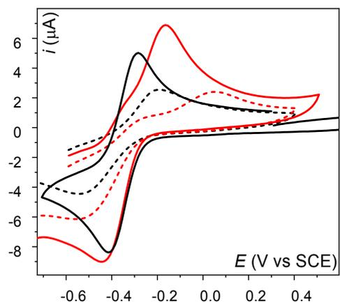
**Figure S2:** Variation of the temperature in  $\text{CH}_2\text{Cl}_2$ . CVs of  $0.5 \text{ mM Mn}^{\text{III}}(\text{TPP})\text{Cl}$  on a  $0.3 \text{ cm}$  glassy carbon electrode in a  $0.1 \text{ M TBAPF}_6/\text{CH}_2\text{Cl}_2$  solution, under Ar at  $298\text{K}$  (black trace), at  $253 \text{ K}$  (black dashed trace) and under  $\text{O}_2$  at  $298 \text{ K}$  (red trace) and at  $253 \text{ K}$  (red dashed trace).
