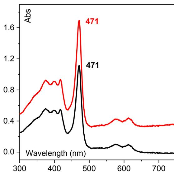
**Figure S3:** UV-vis spectrum of  $0.1 \text{ mM Mn}^{\text{III}}(\text{TPP})\text{Cl}$ , at  $298 \text{ K}$ , in  $0.2 \text{ M TBAPF}_6/\text{CH}_2\text{Cl}_2$ . Under Ar (red trace) and under  $\text{O}_2$  (black trace).
