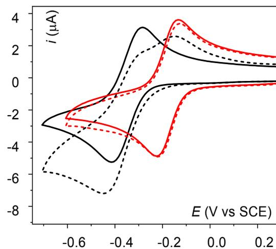
**Figure S6:** CVs of 0.5 mM  $\text{Mn}^{\text{III}}(\text{TPP})\text{Cl}$  at 298 K on a 0.3 cm glassy carbon electrode under Ar in a 0.1 M  $\text{TBAPF}_6$  / $\text{CH}_2\text{Cl}_2$  (black trace) or / DMF (red trace) and under  $\text{O}_2$  in a 0.1 M  $\text{TBAPF}_6$  / $\text{CH}_2\text{Cl}_2$  (dashed black trace) or / DMF (dashed red trace)
