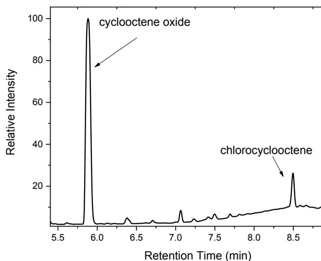
**Figure S15:** Chemical oxidation of cyclooctene using a modified literature procedure.<sup>4</sup> Stirring of two hours of the following biphasic system. Organic phase: 1 ml of Dichloromethane with 13 mM of MnTPPCI, 26 mM of TBACI as a surface factor, 0.2 M of cyclooctene. Aqueous phase: 2 ml of sodium hypochlorite solution 10 % w/w. Chromatogram obtained of the organic phase after removing the catalyst on a small silica column. Both oxidation and chlorination products are observed.
