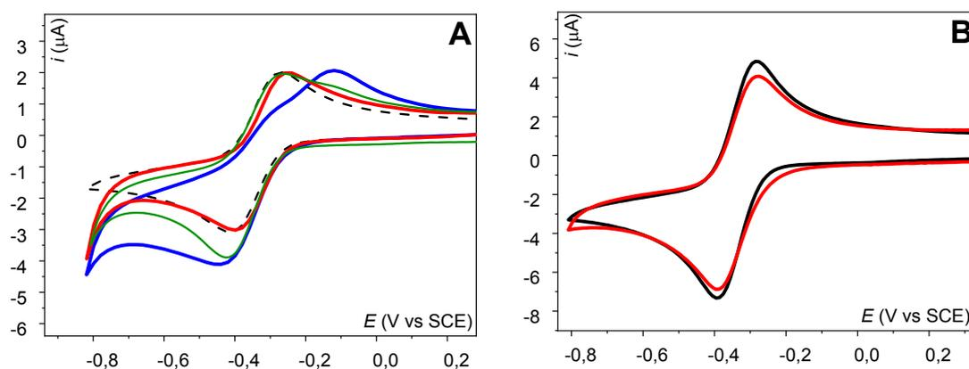
**Figure S9:** CVs of 0.5 mM  $\text{Mn}^{\text{III}}(\text{TPP})\text{Cl}$  in 0.1 M  $\text{TBAPF}_6/\text{CH}_2\text{Cl}_2$  on a 0.3 cm glassy carbon electrode, at 298 K. **A:** Under Ar (black trace), under  $\text{O}_2$  (blue trace), under  $\text{O}_2$  with 20 mM of 1-Melm (red trace) or with 5 mM of TBACl (green trace). **B:** Under Ar (black trace) and under Ar with 440 mM of anhydride (red trace).
