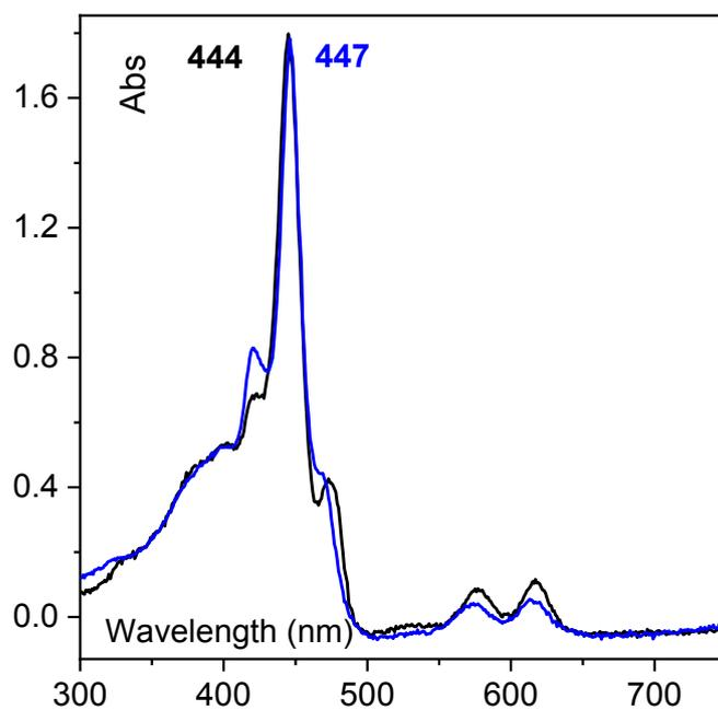
**Figure S5:** UV-vis spectrum of 0.1 mM Mn<sup>III</sup>(TPP)Cl, at 298 K, in 0.2 M TBAPF<sub>6</sub>/CH<sub>2</sub>Cl<sub>2</sub> after 10 min at E<sub>app</sub> = -0.45 V vs SCE. Under Ar (black trace) and under O<sub>2</sub> (blue trace). The optical path for the experiment under Ar was 0.2 cm. The intensities are normalized and the baseline of the spectra is corrected.
