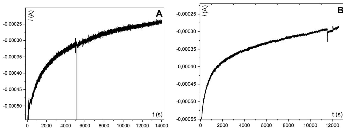
**Figure S10:**  $i(\text{A})$  vs  $t(\text{s})$  plot of preparative scale electrolysis at 298 K of a 0.5 mM solution of  $\text{Mn}^{\text{III}}(\text{TPP})\text{Cl}$  in 0.1 M  $\text{TBAPF}_6/\text{CH}_2\text{Cl}_2$  under  $\text{O}_2$  in presence of 0.44 M of anhydride. **A)** and with 40 mM of 1-Melm (faradaic efficiency for cyclooctene oxide 81%). **B)** and with 5 mM of TBACl with  $E_{\text{app}} = -0.45$  V for 4 hours (faradaic efficiency for cyclooctene chloride 53%)
