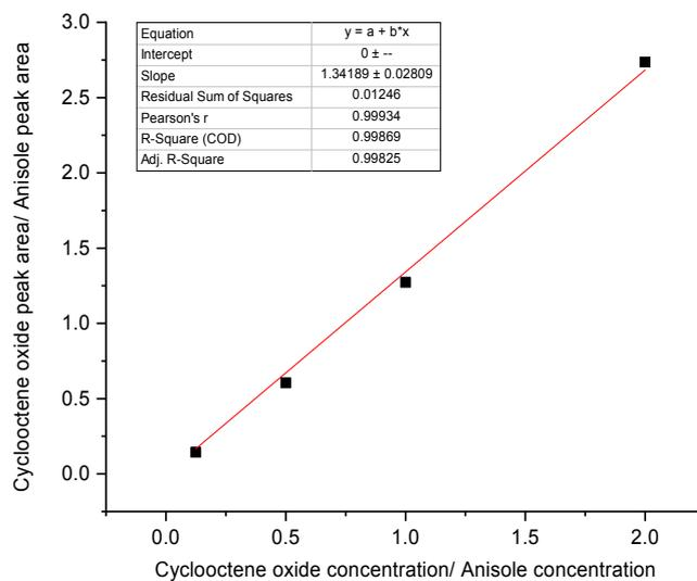
**Figure S14:** Calibration curve for cyclooctene oxide. The internal standard used was anisole. The concentration of the latter was 2 mM on every sample. The concentrations of cyclooctene were: 0.25 mM, 1 mM, 2 mM and 4 mM.
