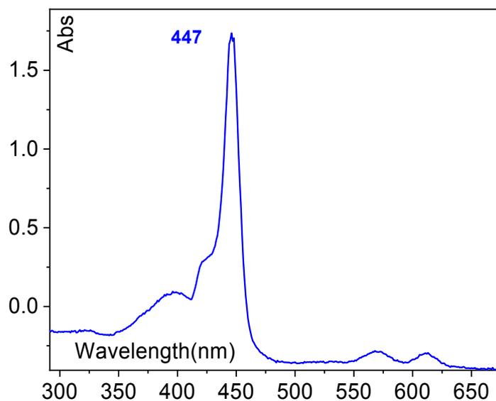
**Figure S4:** UV-vis spectrum of 0.1 mM Mn<sup>III</sup>(TPP)Cl, at 253 K, in 0.2 M TBAPF<sub>6</sub>/CH<sub>2</sub>Cl<sub>2</sub> under O<sub>2</sub> and at E<sub>app</sub> = -0.45 V vs SCE.
