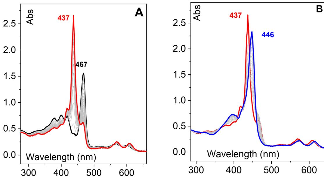
**Figure S8:** UV-vis spectrum of 0.1 mM Mn<sup>III</sup>(TPP)Cl, at 253 K, in 0.2 M TBAPF<sub>6</sub> / DMF under O<sub>2</sub>. **A)** Starting Mn<sup>III</sup> complex (black trace) and after 10 min at -0.45 V (red trace). **B)** Evolution (from red trace to blue trace) after 10 min at -1.1 V vs SCE.
