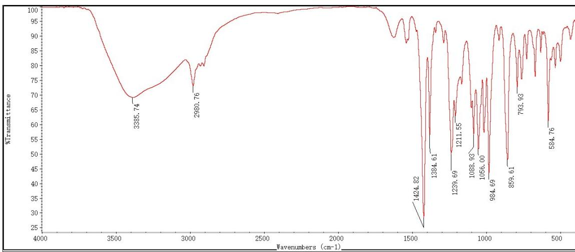
**Fig. S13** FT-IR spectrum of **3** (KBr, cm<sup>-1</sup>)
