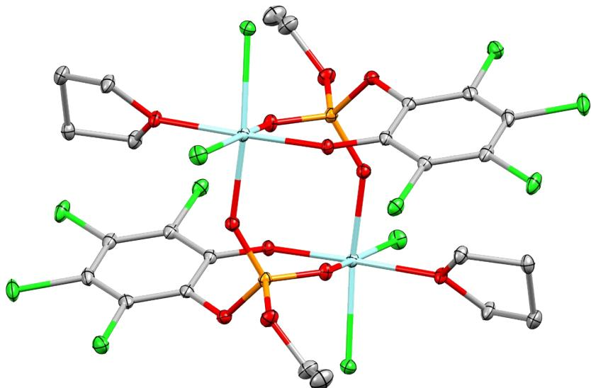
**Fig. S1** Thermal ellipsoid plot for **2** with the anisotropic displacement parameters depicted at the 30% probability level. Hydrogen atoms are omitted for clarity.
