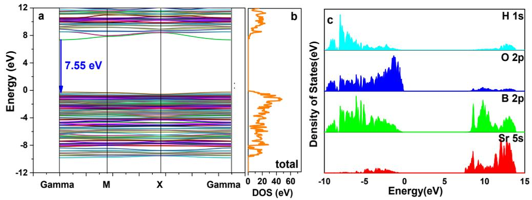
**Figure S3.** The energy band structure, total and partial density of states of SBH calculated based on the HSE06 functional.
