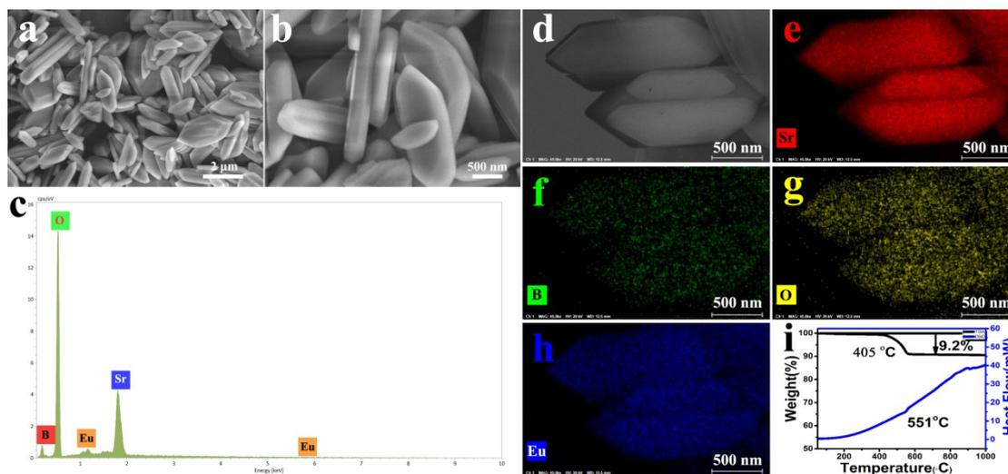
**Figure S2.** (a, b, and d) SEM images, (c) EDS pattern, (e, f, g, and h) corresponding element mapping images and (i) TG-DSC of  $\text{SBH}:\text{Eu}^{2+}$ .
