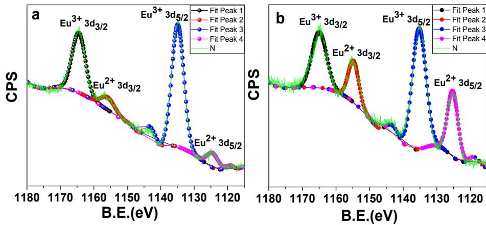
**Figure S4.** (a) High-resolution XPS spectra and (b) the ion sputter depth profiling high-resolution XPS of Eu  $3d_{3/2}$  and Eu  $3d_{5/2}$  in SBH:Eu $^{2+}$ .
