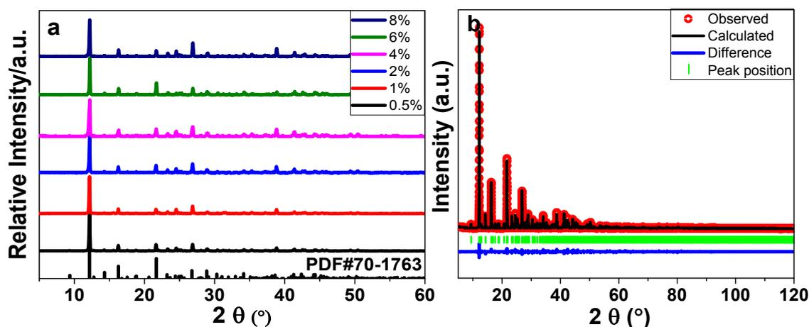
**Figure S1.** (a) XRD patterns of  $\text{SBH}:\text{xEu}^{2+}$  ( $0.5\% \leq x \leq 8\%$ ), and standard patterns of PDF card No. 70-1763 for  $\text{Sr}[\text{B}_8\text{O}_{11}(\text{OH})_4]$ ; (b) Rietveld refinement XRD patterns of SBH. The measured data, fitting data, and their difference are depicted with red circles, black solid line, and blue solid line, respectively. The green short vertical lines show the positions of Bragg reflections of the fitting XRD patterns.
