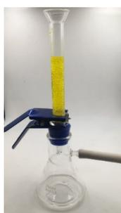
**Fig. S7** A dead-end filtration cell for evaluate the catalytic performance of MR.
