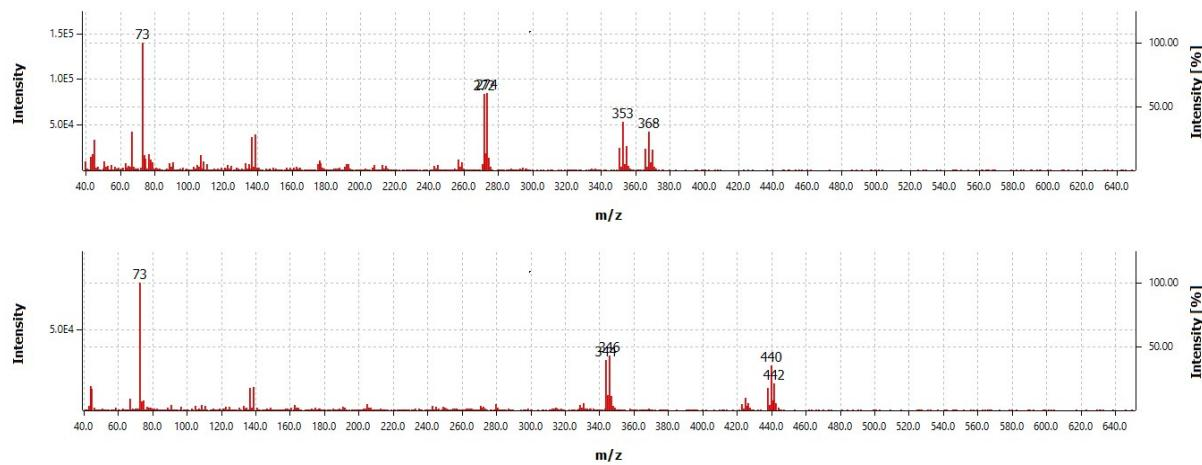
The right-hand side of the peak at 9.49 min ( $m/z$  288) contains a second product at  $m/z$  360. This matches the peak in the next aliquot at 9.52 min and therefore two species are overlapping above:
