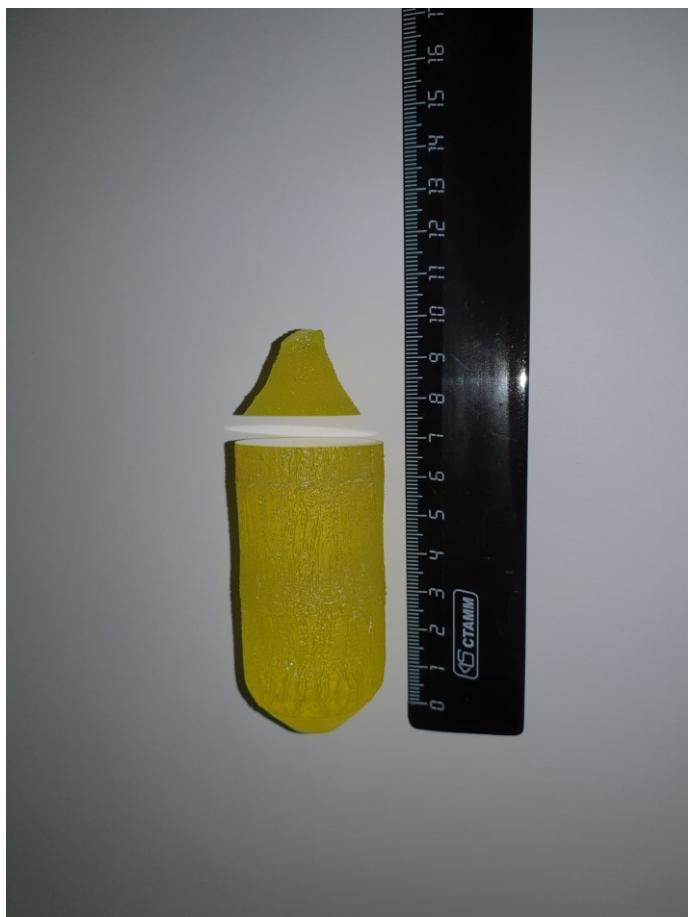
Figure S1. Example photo of the grown Ce-doped  $\text{Gd}_3\text{Al}_{2.3}\text{Ga}_{2.7}\text{O}_{12}$  single crystal.
