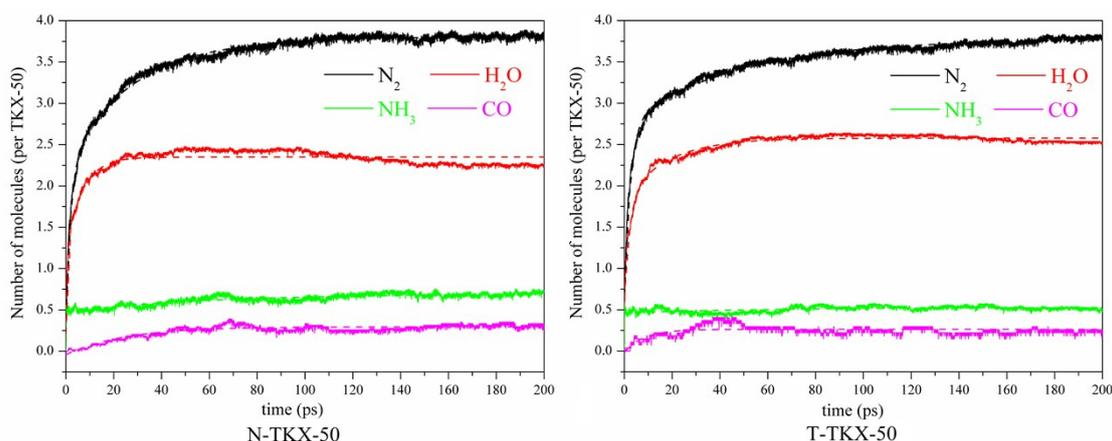
**Fig. 3** Evolutions of the numbers of  $N_2$ ,  $H_2O$ ,  $NH_3$  and  $CO$  molecules (solid lines) and their corresponding fitted curves (dash lines) of N-TKX-50 and T-TKX-50 at 2000 K.
