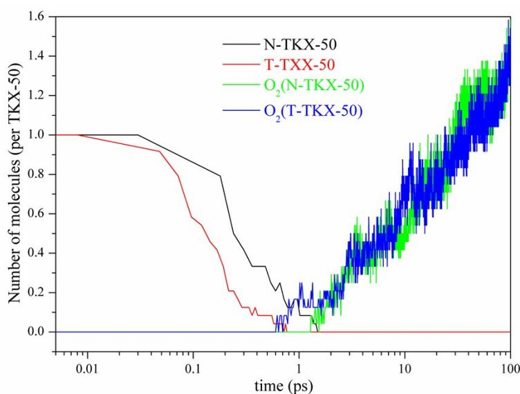
**Fig. 4** TKX-50 distribution and consumption rate of  $O_2$
