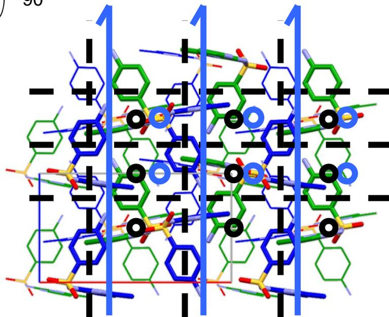
The symmetry elements shown in black apply to the whole structure; those shown in blue apply to the layer only. The offset between the two, mostly along **a**, means that the approximate layer symmetry cannot describe the 3-D structure.
