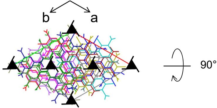
Overlay by translation of the four independent layers (001) after rotation of layers B1 and B2 by 180° around the layer normal
