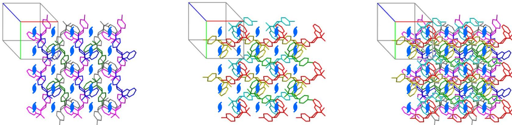
Projections along  $\mathbf{c}^*$  with part of the molecule deleted to show that there is no fourfold axis and that  $\mathbf{c}^*$  is close to  $[1\ 1\ 2]$ , along which the structure is periodic
