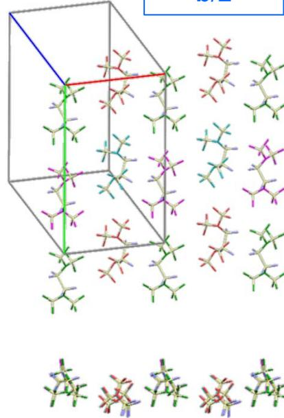
Layer B has a  $b/2$  pseudotranslation; layer A does not. Both layers have crystallographic inversion centers; layer B also has approximate inversion centers.
