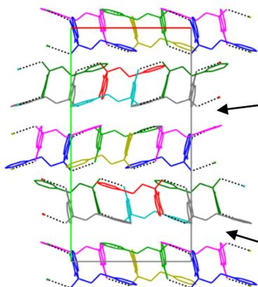
No  $2_1$  axis or glide is possible between layers because there is enantiomeric alternation on both sides of the layer interface
