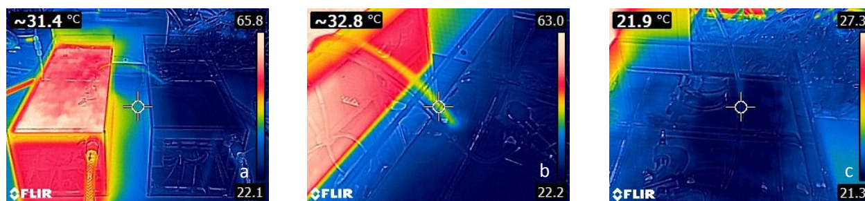
Figure S1. Thermal images of the a) two water baths at different temperatures b) the connecting tube entering the cold bath and c) the tube leaving the cold bath.
