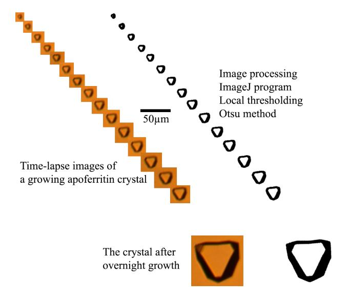
**Figure S1.** Example of time-lapse images of a single progress of crystal growth (left). The result from the image processing is shown in the right. A local thresholding is chosen, because it makes the image processing insensitive to cropping or presence of pixel inhomogeneity outside the very image of the crystal. The Otsu thresholding method is chosen, because its result appears to be in the best conformity with the eye perception.
