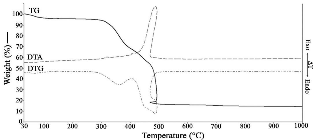
**Fig. S14.** TG, DTG and DTA curves of compound 4
