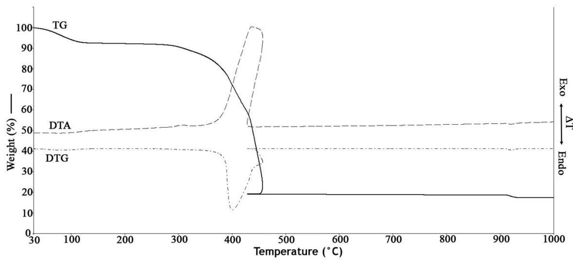
**Fig. S11.** TG, DTG and DTA curves of compound 1
