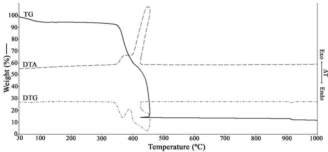
**Fig. S13.** TG, DTG and DTA curves of compound 3
