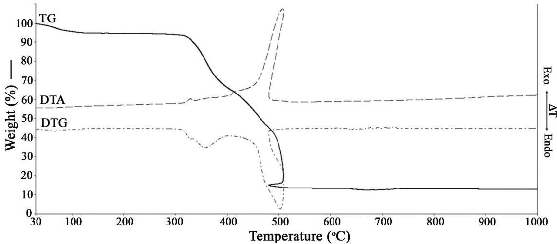
**Fig. S12.** TG, DTG and DTA curves of compound 2
