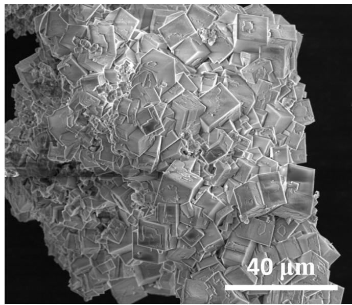
Fig. S1 SEM of KNiF<sub>3</sub> crystals with inter-connected blocks in hydrothermal condition.
