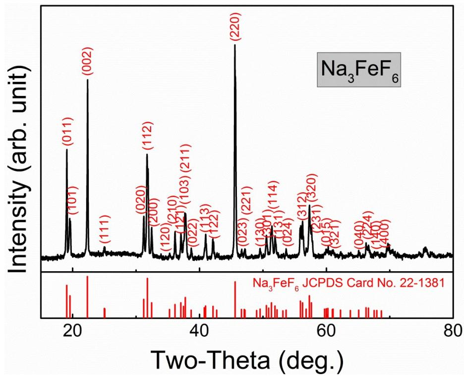
Fig. S17  $\text{Na}_3\text{FeF}_6$  phase was obtained rather than perovskite  $\text{NaFeF}_3$  phase as intended in the same synthetic procedure of hydrothermal route.
