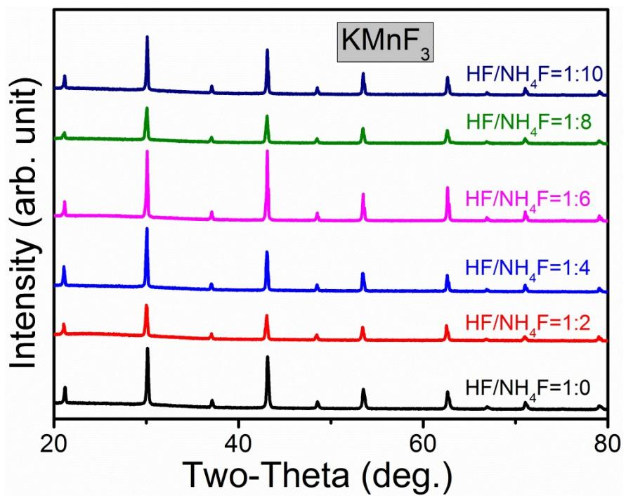
Fig. S6 XRD of  $\text{KMnF}_3$  samples synthesized via hydrothermal method with varied  $\text{HF}/\text{NH}_4\text{F}$  ratio.
