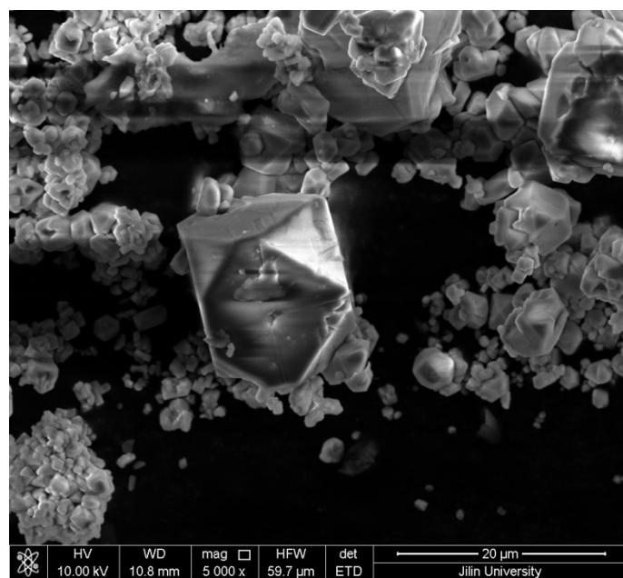
Fig. S10 SEM graph of KFeF<sub>3</sub> synthesized via hydrothermal method with the ratio of HF/NH<sub>4</sub>F is 1:4.
