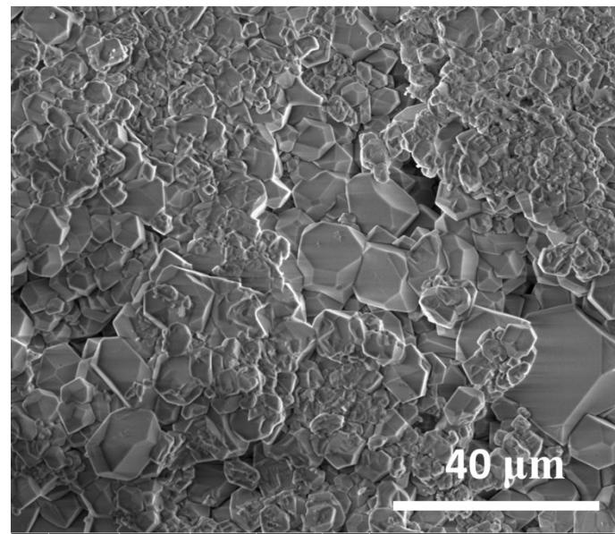
Fig. S3 SEM graph of aggregated KZnF<sub>3</sub> crystals in high concentration of reactants in hydrothermal condition.
