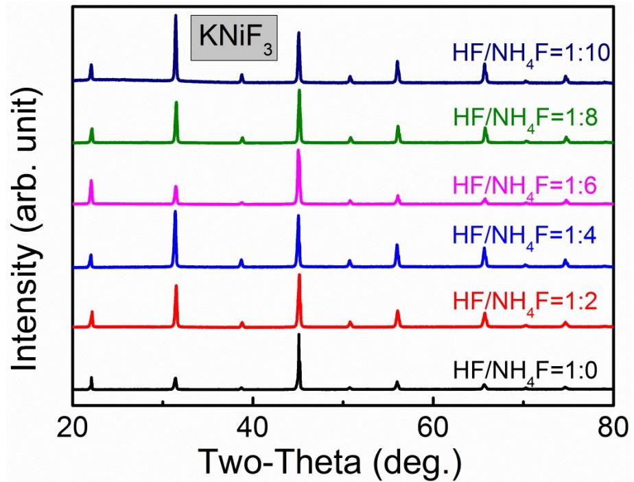
Fig. S8 XRD of KNiF<sub>3</sub> samples synthesized via mild hydrothermal method with tuneable HF/NH<sub>4</sub>F ratio from 1:0 to 1:10.
