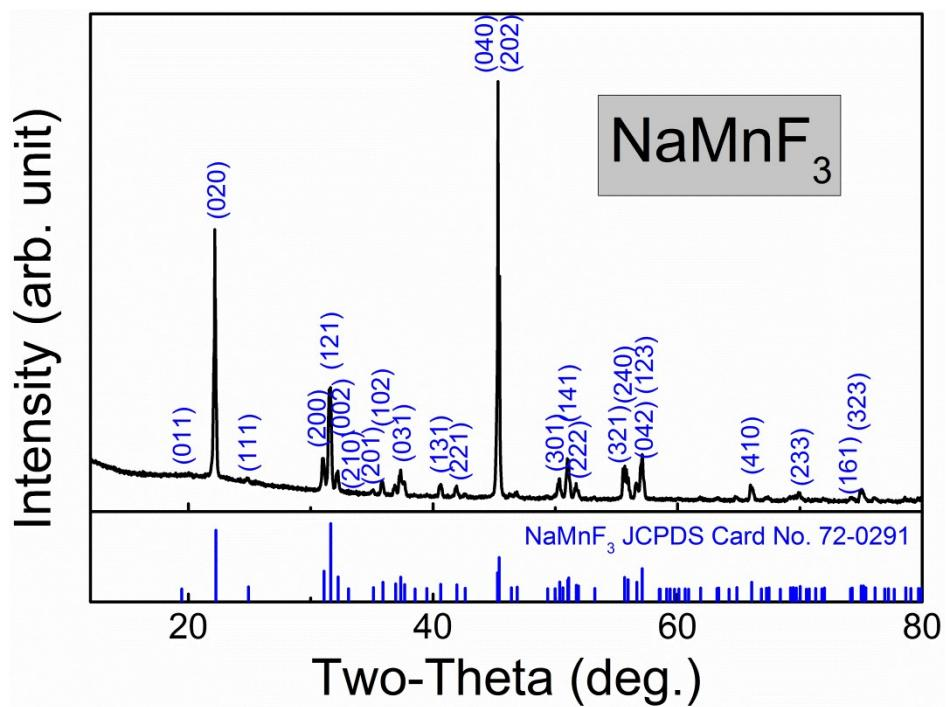
Fig. S13 XRD of  $\text{NaMnF}_3$  sample that crystallized into Pnma space group with the JCPDS Card No. 72-0291.
