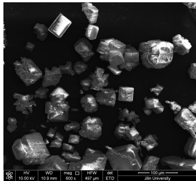
Fig. S14 SEM graph of NaMnF<sub>3</sub> synthesized via mild hydrothermal method, respectively.
