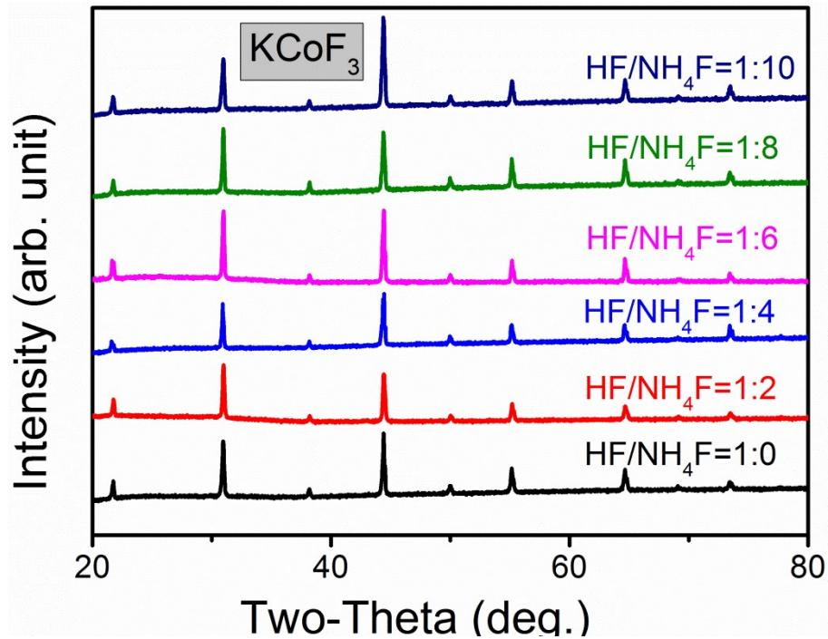
Fig. S7 XRD of  $\text{KCoF}_3$  samples synthesized via mild hydrothermal method with tuneable  $\text{HF}/\text{NH}_4\text{F}$  ratio from 1:0 to 1:10.
