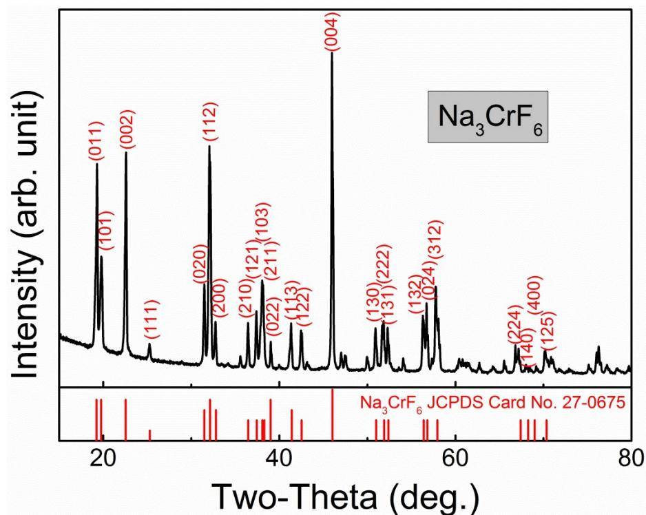
Fig. S16  $\text{Na}_3\text{CrF}_6$  phase was obtained rather than perovskite  $\text{NaCrF}_3$  phase as intended in the same synthetic procedure of hydrothermal route.
