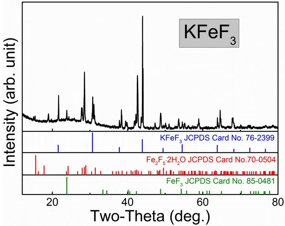
Fig. S11 XRD of  $\text{KFeF}_3$  sample synthesized via similar method of other  $\text{KMF}_3$ . Perovskite phase could be indexed according to the JCPDS Card No. 76-2399, and other impurity phases can be indexed as shown in the red and green bars for  $\text{Fe}_2\text{F}_5 \cdot 2\text{H}_2\text{O}$  (JCPDS Card No. 70-0504) and  $\text{FeF}_3$  (JCPDS Card No. 85-0481), respectively.
