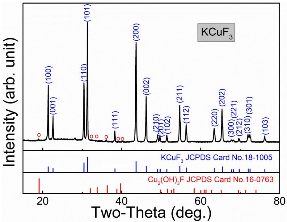
Fig. S12 XRD of hydrothermally synthesized  $\text{KCuF}_3$  sample with  $\text{Cu}_2(\text{OH})_3\text{F}$  impurity phase. Open circle and red bars indicate the diffraction peak positions in the data.
