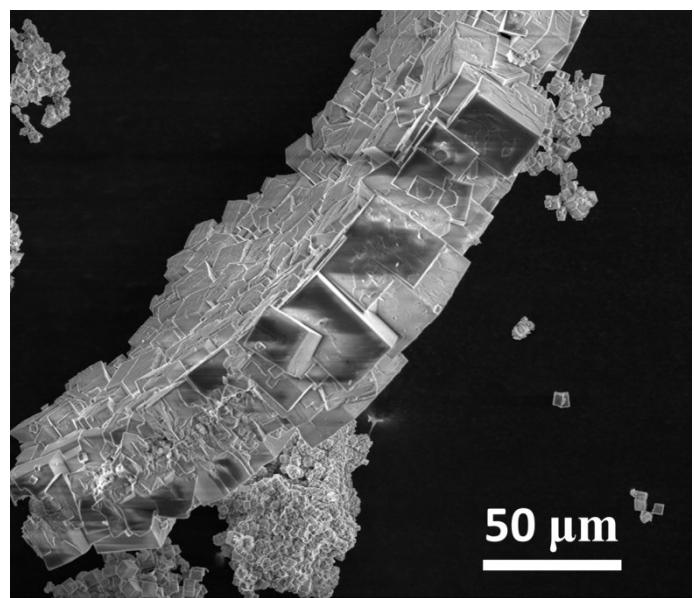
Fig. S2 SEM of KNiF<sub>3</sub> crystals with inter-locked mats in hydrothermal condition.
