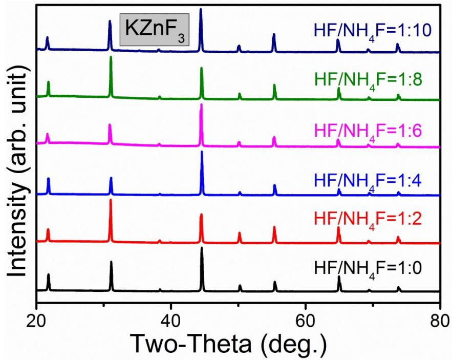
Fig. S9 XRD of KZnF<sub>3</sub> samples synthesized via mild hydrothermal method with tuneable HF/NH<sub>4</sub>F ratio from 1:0 to 1:10.
