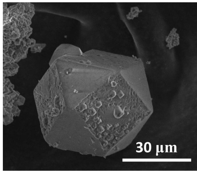
Fig. S4 SEM graph of KZnF<sub>3</sub> with small sized twin crystals on the pit at these facets obtained in hydrothermal condition.
