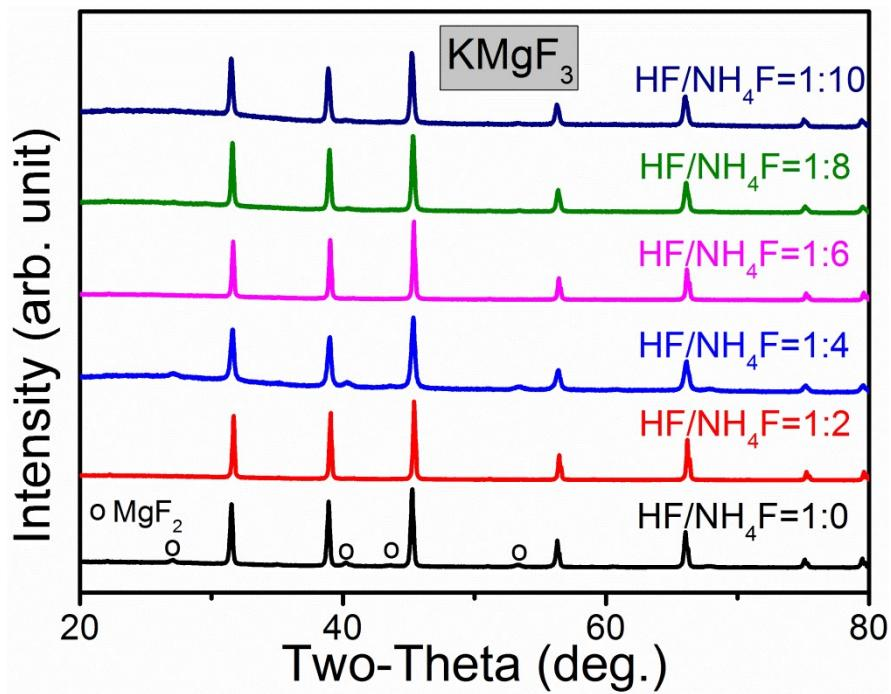
Fig. S5 XRD of hydrothermal synthesized  $\text{KMgF}_3$  crystal with tuneable mineralizer ratio of  $\text{HF}/\text{NH}_4\text{F}$  from 1:0 to 1:10. Black circles in the data of  $\text{HF}/\text{NH}_4\text{F}=1:0$  indicate the diffraction peak positions of  $\text{MgF}_2$  impurity.
