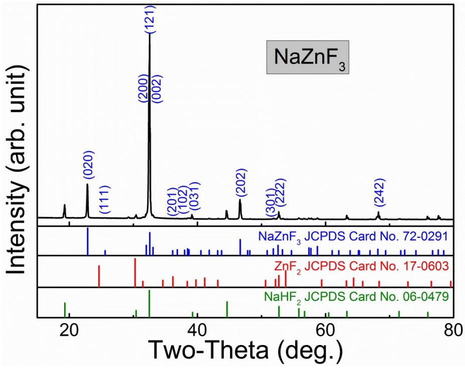
Fig. S15 XRD of  $\text{NaZnF}_3$  sample synthesized via mild hydrothermal method with impurities of  $\text{ZnF}_2$  and  $\text{NaHF}_2$  phases.
