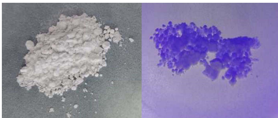
Fig. S10. The photograph of compound 1 before and after under irradiation with a UV-vis light at 365 nm.
