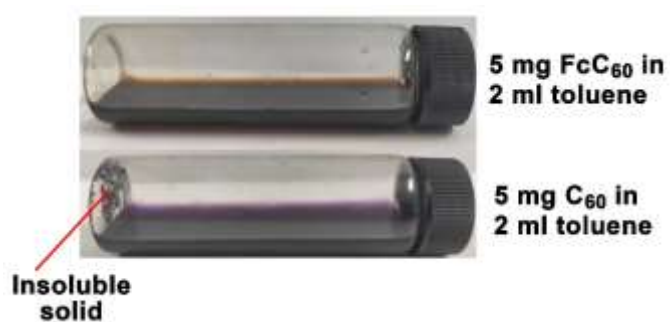
Figure S5. The solubility comparison of C_{60} and FcC_{60} . At the same amount (5 mg) in toluene (2 mL), C_{60} s can not be completely dissolved, while FcC_{60} s are all dissolved.
