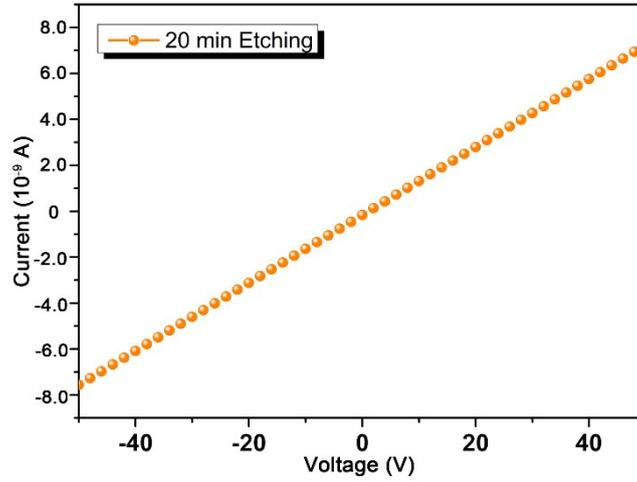
**Figure S2** I-V curve of Au/CdTe contact structure after 20 min chemical etching.
