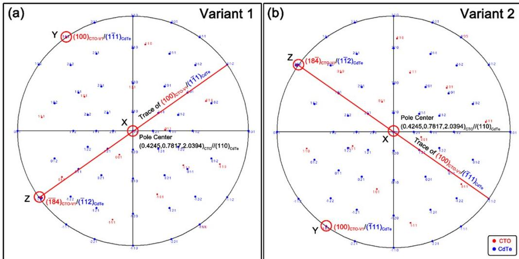
**Figure S5** Stereographic projection of planes for the established orientation relationships between CTO and CdTe: (a) variant 1; (b) variant 2.
