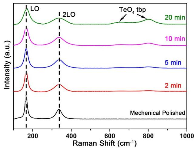
**Figure S4** Raman spectroscopy of CdTe wafers under different surface treatments.
