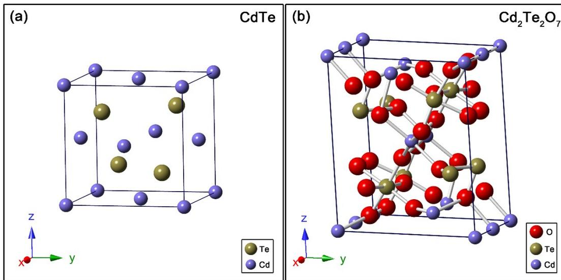
**Figure S3** Structure unit cells of CdTe (a) and  $\text{Cd}_2\text{Te}_2\text{O}_7$  (b).
