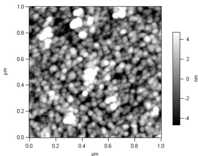
**Figure S1** AFM image of CdTe surface after 20 min chemical etching in 2%  $\text{Br}_2$ -MeOH solution shows no significant change in both surface morphology and roughness when compares with the sample etched for 10 min.
