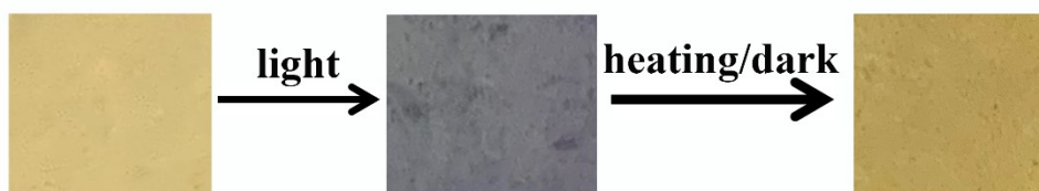
Figure S4 Color changes of the powder samples for 1 upon light and heating/dark treatment.
