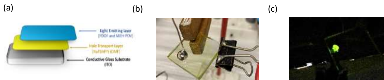
Fig. S11. (a) Schematic of light-emitting diode fabricated using Na(TBAPy)(DMF) as a hole transport layer, (b) photograph of coated substrate connected to a DC power source and (c) photograph of active LED emitting light at 4.45 V (26 mA).
