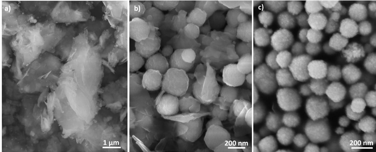
Figure SI.2. SEM micrographs recorded on the powders recovered from the DEG reaction solution after different heating times (the temperature being fixed to 180°C) corresponding to a) the layered hydroxy-acetate cobalt salt alone, b) a mixture of that and the cobalt oxide and c) the cobalt oxide alone.
