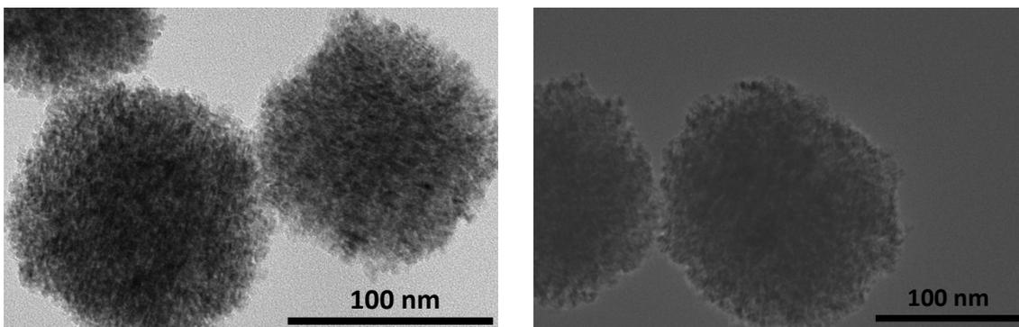
**Figure SI.4.** TEM images of textured sub-micrometer sized CoO particles produced in DEG (left) and in TrEG (right)
