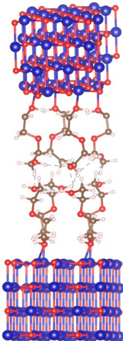
**Figure SI.3.** Illustration of the Hydrogen bonds (see dashed lines) between DEGs adsorbed one two neighbour CoO nanocrystals. (Oxygen atoms appear in red).
