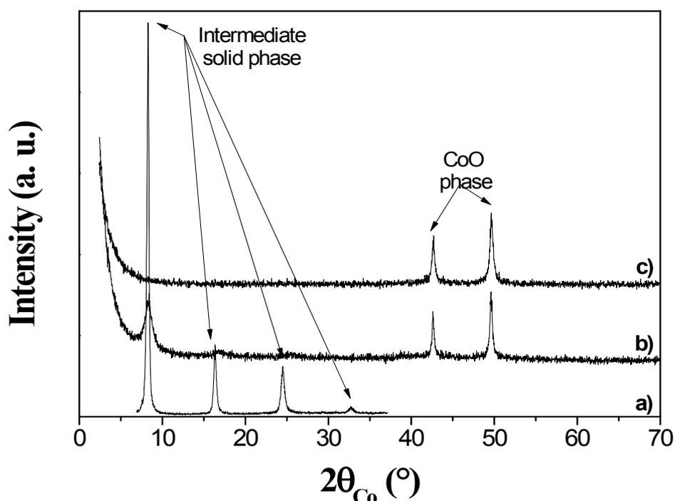
**Figure SI.1.** XRD patterns recorded on the powders isolated from the DEG reaction solution after different heating times (the temperature being fixed to 180°C) and corresponding respectively to a) the layered hydroxy-acetate cobalt salt, b) a mixture of that and the cobalt oxide and c) the cobalt oxide alone.
