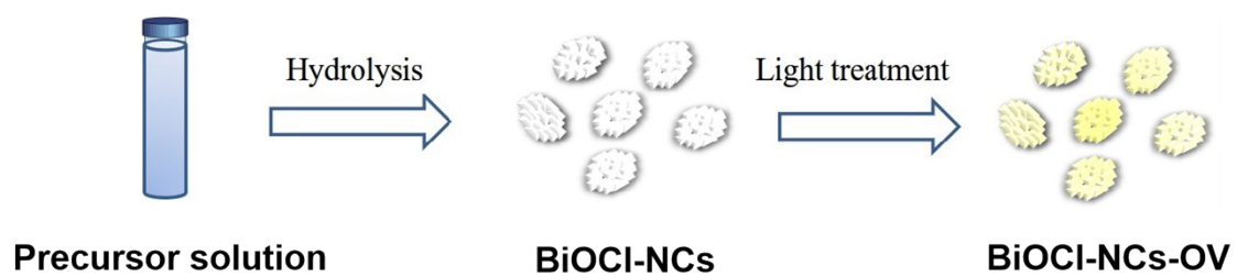
Figure S1. Schematic illustration of the synthesis procedure for the BiOCl-NCs-OV.
