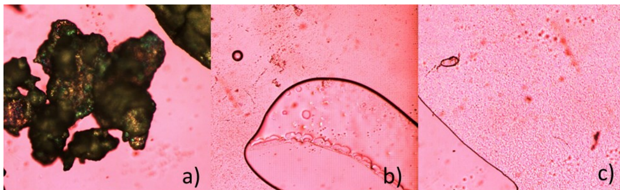
Figure S92: Polarizing optical microscopy images of C_{12}C_1C_4 : a) Cr at 30 °C (1 st heating); b) L_{iso} at 60 °C (1 st heating); c) Cr at 20 °C (2 nd heating)
