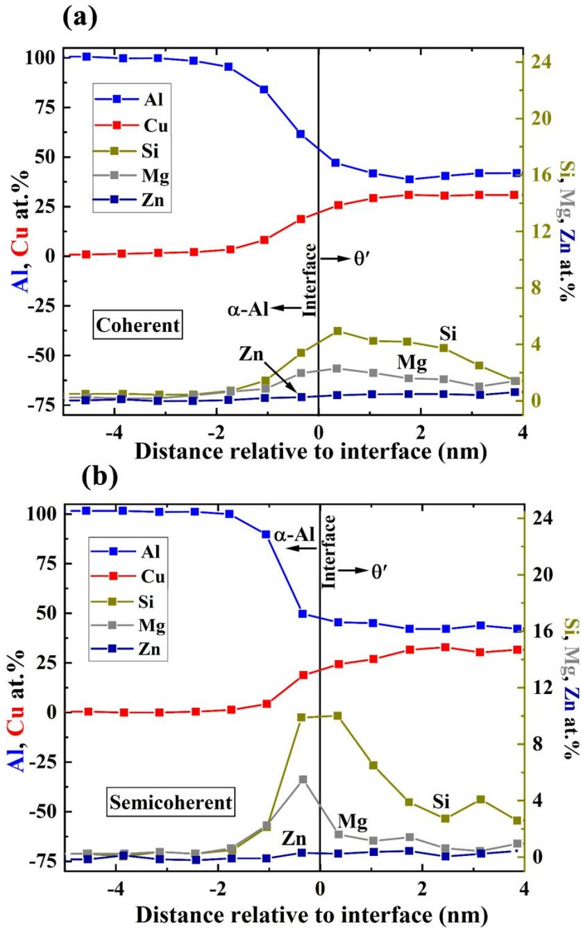
**Fig. S1** Concentrations of Al, Cu, Mg, Si, and Zn as a function of distance from the coherent (a) and semicoherent (b)  $\alpha$ -Al/ $\theta'$  matrix-precipitate interfaces after aging at 463 K for 8 h. Al and Cu levels are identified on the left ordinates; Si, Mg, and Zn levels appear on the right. The location of each interface is depicted with a vertical line. (The data are taken from ref. <sup>1</sup>)
