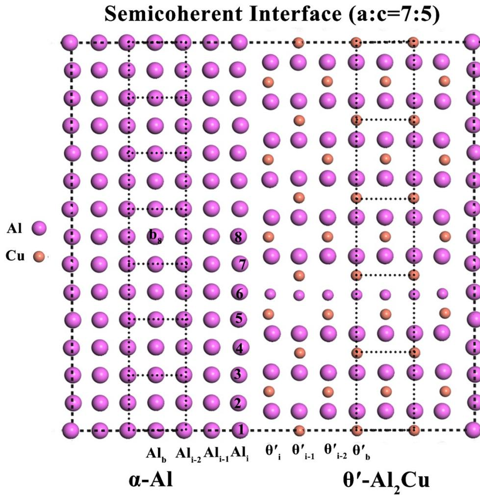
**Fig. S6** Supercell slab models to simulate the segregation energies of Si (Mg) in the  $(010)_{\text{Al}} \parallel (010)_{\theta'}$  semicoherent interface with a mismatch of 2.29% utilizing LCAO. Large and small spheres represent Al and Cu atoms. Dashed lines mean the  $7a_{\text{Al}}=5c_{\theta'}$  relationships of the semicoherent interface. The numbers from 1 to 8 represent the substitutional sites for solutes in the  $\text{Al}_i$  layer.
