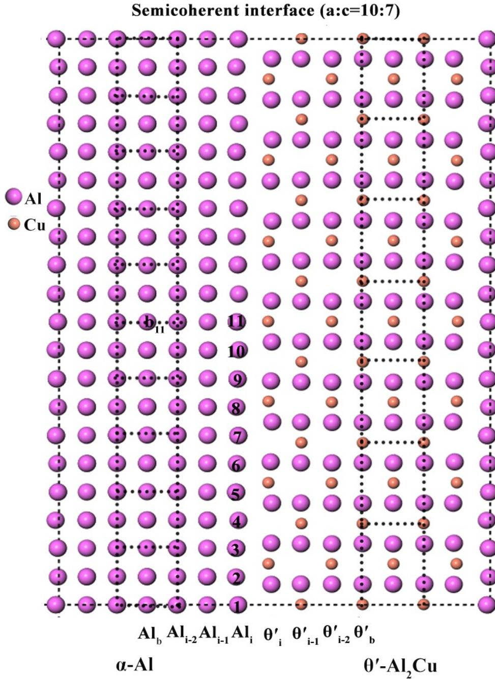
**Fig. S7** Supercell slab models to simulate the segregation energies of Si (Mg) in the  $(010)_{\text{Al}} \parallel (010)_{\theta'}$  semicoherent interface with a mismatch of 0.25% utilizing LCAO. Large and small spheres represent Al and Cu atoms. Dashed lines mean the  $10a_{\text{Al}}=7c_{\theta'}$  relationships of the semicoherent interface. The numbers from 1 to 11 represent the substitutional sites for solutes in the  $\text{Al}_i$  layer.
