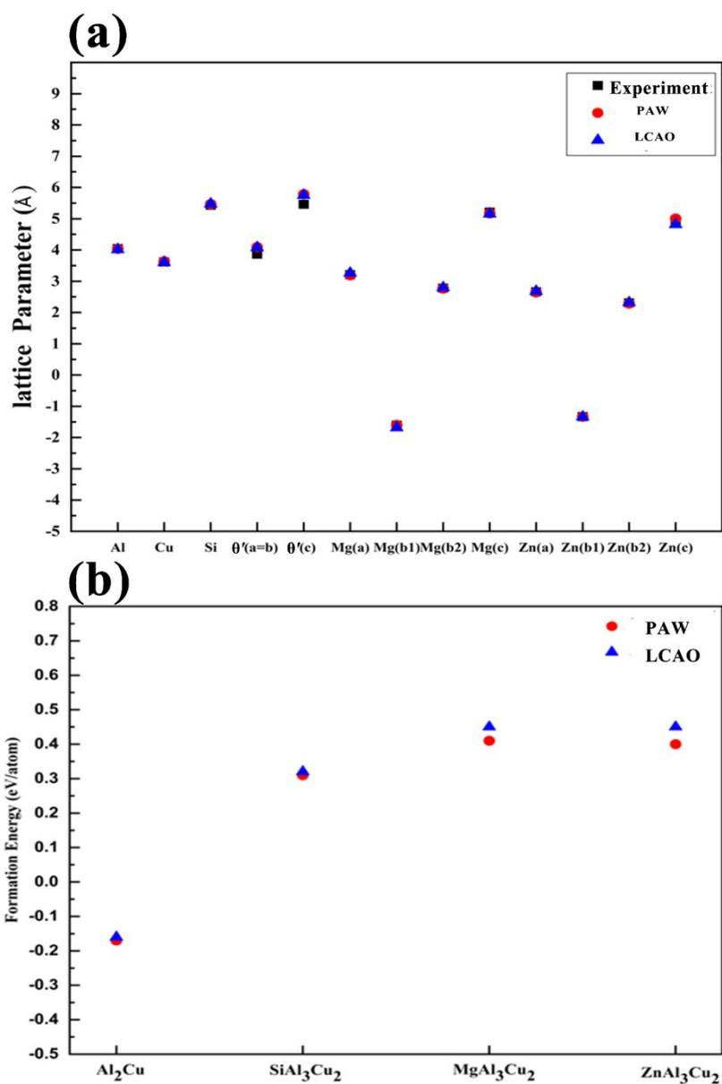
**Fig. S2** Calculated lattice parameters of bulks [Al, Cu,  $\text{Al}_2\text{Cu}$  ( $a=b$ ), Si, Mg ( $a$ ,  $b_1$ ,  $b_2$ ,  $c$ ), Zn ( $a$ ,  $b_1$ ,  $b_2$ ,  $c$ )] (a) and formation energy for  $\text{XAl}_3\text{Cu}_2$  ( $X=\text{Si}$ , Mg, Zn) using LCAO (blue triangles) and PAW (red circles) (b).
