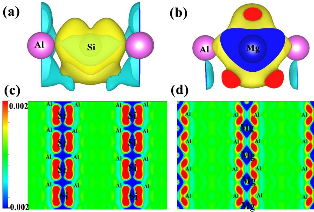
**Fig. S4** 3D and contour on the (001) plane of charge density difference of Si (a, c) and Mg (b, d) at the Al<sub>i</sub> layer (Fig. 2b) in the Al/Al<sub>2</sub>Cu semicoherent interface using PAW. (The isosurface value is 0.002 eV/bohr<sup>3</sup>). Yellow and green regions denote charge accumulation and depletion, respectively.
