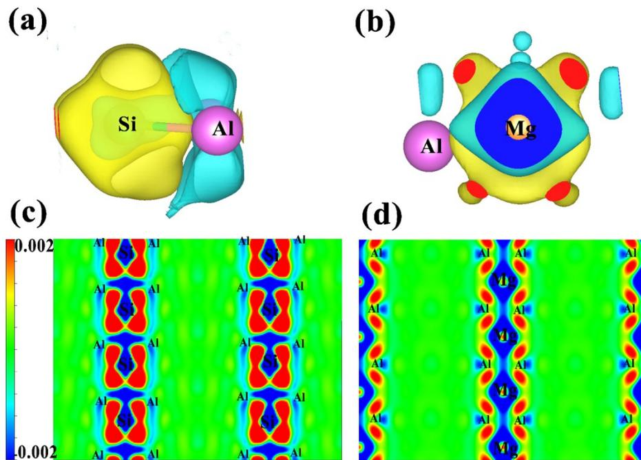
**Fig. S5** 3D and contour on the (001) plane of charge density difference of Si (a, c) and Mg (b, d) at Al<sub>i</sub> layer (Fig. 2b) in the Al/Al<sub>2</sub>Cu semicoherent interface by further relaxing the LCAO output lowest energy structures using PAW. (The isosurface value is 0.002 eV/bohr<sup>3</sup>). Yellow and green regions denote charge accumulation and depletion, respectively.
