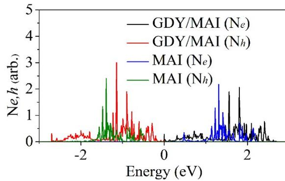
**Fig. S4** The number of photogenerated electrons and holes on the energy level  $E$  in the MAI-terminated system.
