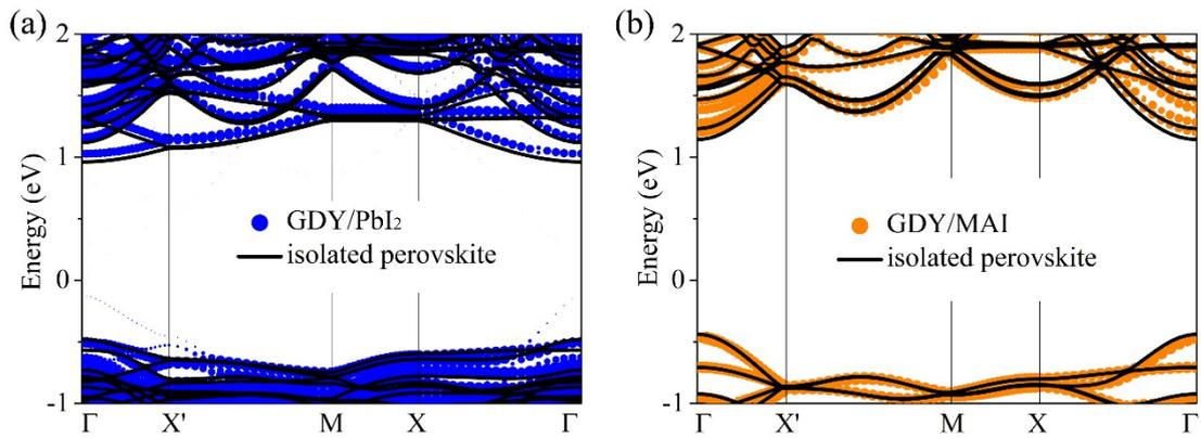
**Fig. S2** Projected band structure of perovskite slab in the GDY/PbI<sub>2</sub> (a) and the GDY/MAI (b) heterostructures compared to isolated perovskite slab. The size of the symbol indicates the contribution weight.
