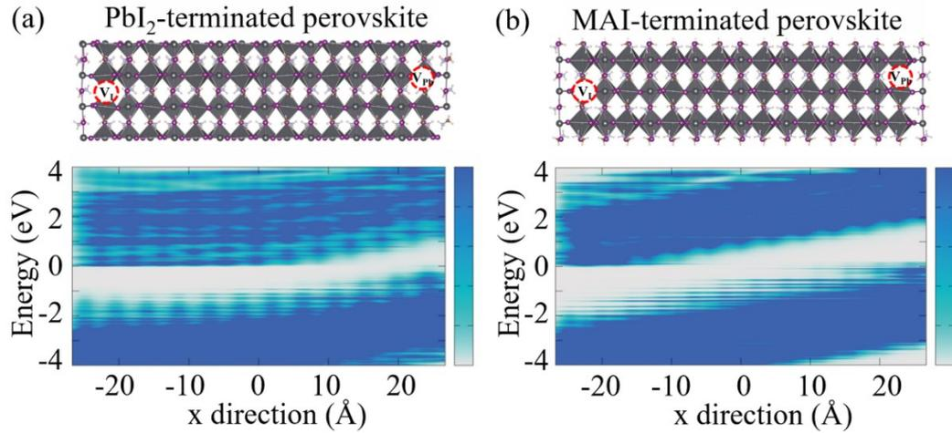
**Fig. S3** (a) The structure of p-n heterojunction (top panel) and the LDOS in transport direction (bottom panel) of  $\text{PbI}_2$ -terminated surface; (b) The structure of p-n heterojunction (top panel) and the LDOS in transport direction (bottom panel) of MAI-terminated surface.
