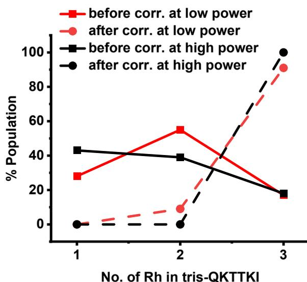
Fig. SI.3. Correction for prebleaching on the population obtained from standard tris-Rh-QKTTKI peptide as a function of laser power 0.7 mW (shown in red) and 1.47 mW (shown in black). Solid-squares and circles represent population before and after correction respectively at the two powers.
