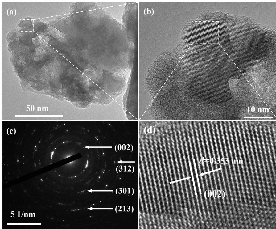
Fig. S2 Microstructures of the  $\text{Cu}_{3+\delta}\text{In}_5\text{Te}_9$  ( $\delta=0.1$ ) powder sample. (a) TEM image; (b) Zoomed view in (a); (c) Corresponding selected area electron diffraction (SAED) pattern; (d) Magnified image of (b), the  $d$  spacing between (002) planes is 0.353 nm.
