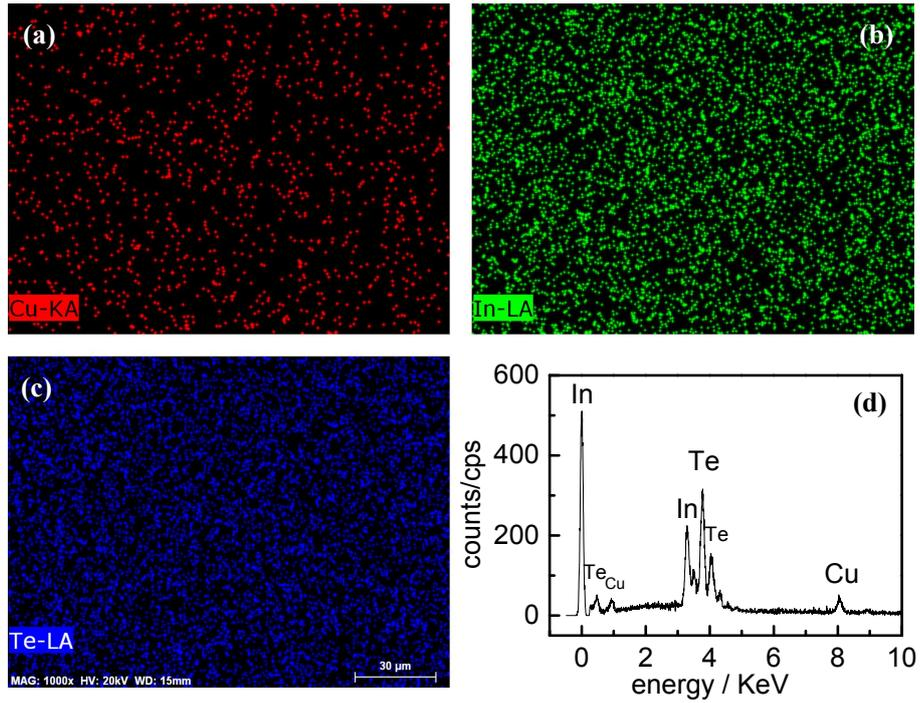
Fig.S1 EPMA mappings of three elements on polished sample  $\text{Cu}_{3.1}\text{In}_5\text{Te}_9$  surface (a) Cu, (b) In, (c) Te, (d) an EDAX pattern.
