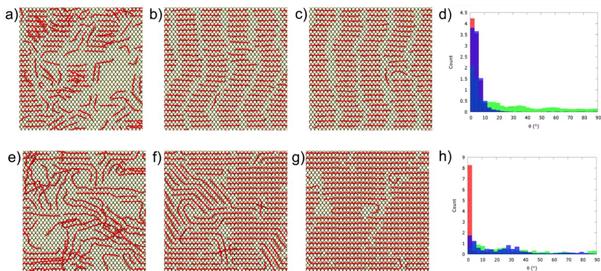
**Figure S4.** Configuration of C15 (top) and C45 (bottom) alkane chain aggregates on phosphorene as cast (a,e), and equilibrated in kinetic (b,f) and thermodynamic (c,g) conditions. Distribution of the angular parameter (d,h) for aggregates as cast (green bars), in kinetic (blue bars) and thermodynamic (red bars) conditions.
