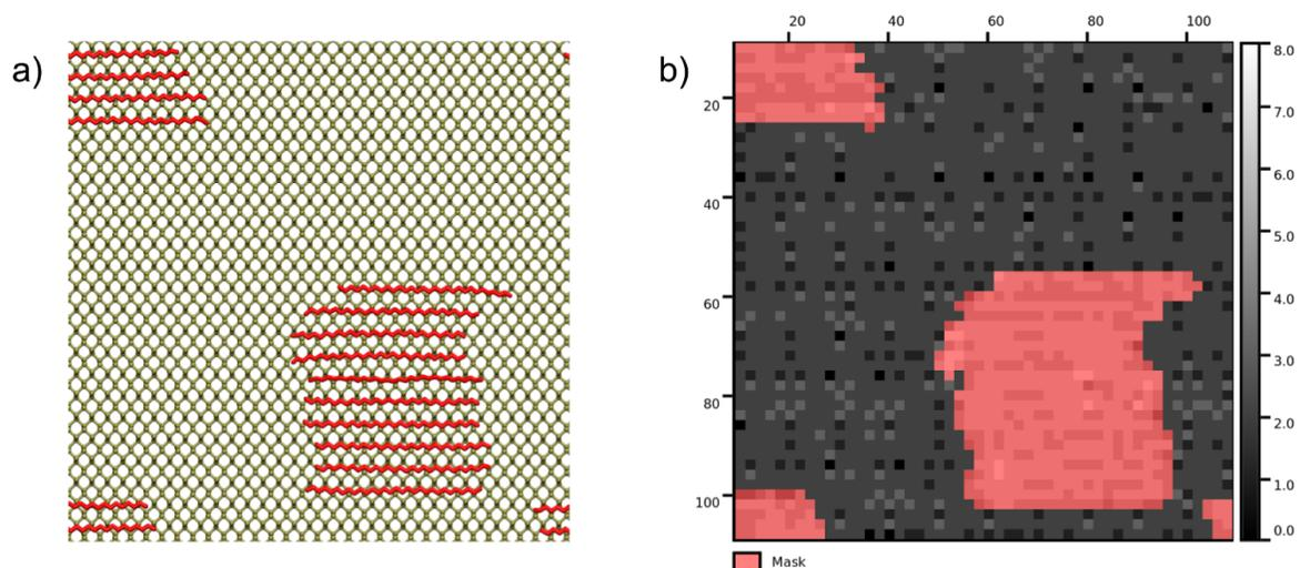
**Figure S1.** Determination of the surface area of phosphorene covered by alkane chains. The configuration obtained by MD (a) is first discretized by convolution with a van der Waals sphere with radius 2 Å and the covered surface area is computed by selecting all regions with an height that is higher than 4 Å with respect to the phosphorene surface.
