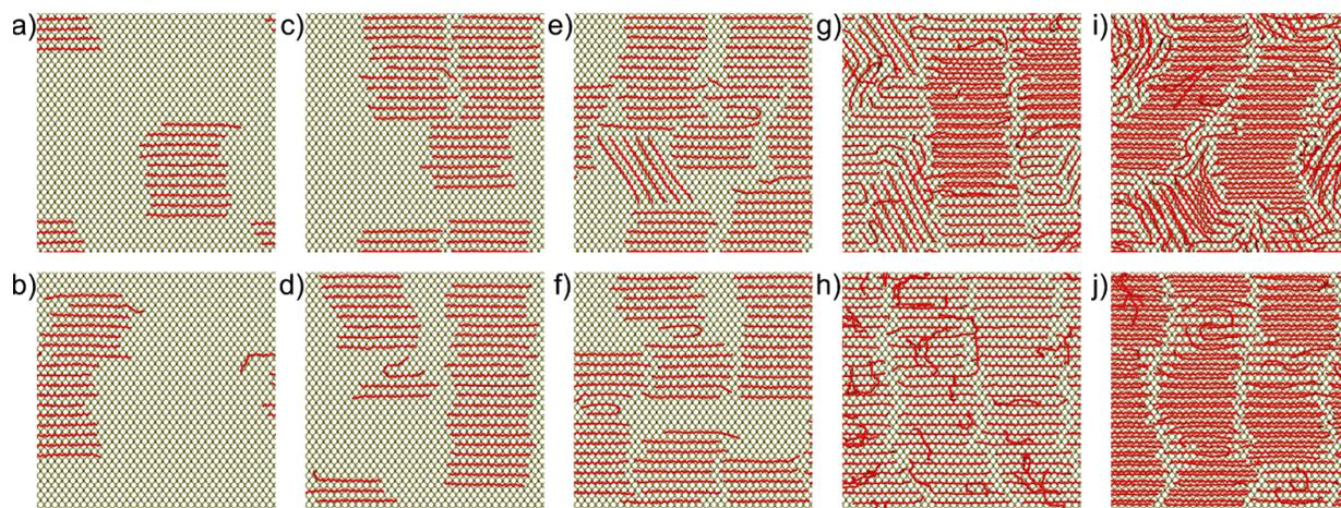
**Figure S2.** Equilibrated structures of C30 aggregates on phosphorene grown in kinetic (top) and thermodynamic (bottom) conditions, as a function of the coverage (a, b:  $\Theta=0.25$ ; c, d:  $\Theta=0.50$ ; e, f:  $\Theta=0.75$ ; g, h:  $\Theta=1.50$ ; i, j:  $\Theta=2.00$ ).
