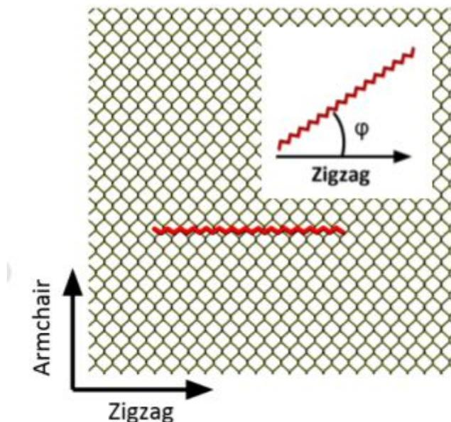
**Figure S6.** Configuration used for the evaluation of the interaction energies for single alkane chains on a phosphorene monolayer at the DFT level. Calculations were performed for C12 and C24 alkanes, as indicated in the Computational Details sections, including the Grimme correction (DFT-D3) for dispersion forces (J. Chem. Phys. 132, 154104 (2010)).
