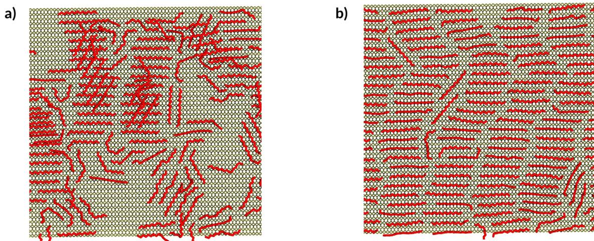
**Figure S3.** Configuration of C30 grown on a phosphorene layer model of about 10x10 nm at the nominal coverage  $\Theta=1.0$  in strongly (interval of 10ps between insertion of new molecules) kinetically-controlled conditions a) before and b) after annealing at 400K for 20 ns and further equilibration at 300K for 10 ns.
